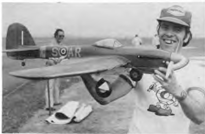
Left: Peter Miller from Glasgow has given his entry in the Novice Stunt the 'Typhoon' look. It's Enya 45 powered, weighs 48ozs. and, believe it or not, is tissue covered although beautifully finished with rivets and panel lines on the camouflage. Right: Winner of the Gold Trophy, Bill Draper and his Super Hawk. Plans in Aeromodeller soon!
