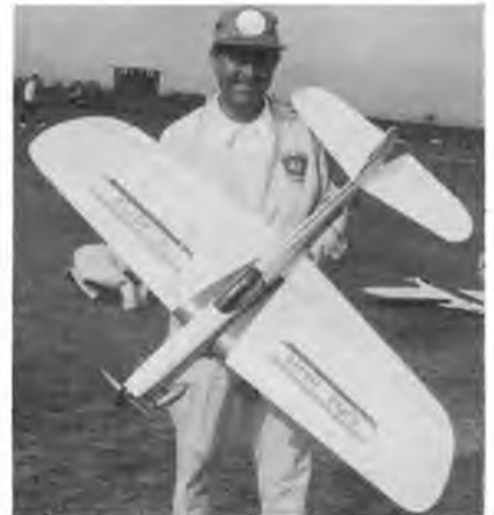
Left: Peter Miller from Glasgow has given his entry in the Novice Stunt the 'Typhoon' look. It's Enya 45 powered, weighs 48ozs. and, believe it or not, is tissue covered although beautifully finished with rivets and panel lines on the camouflage. Right: Winner of the Gold Trophy, Bill Draper and his Super Hawk. Plans in Aeromodeller soon!
