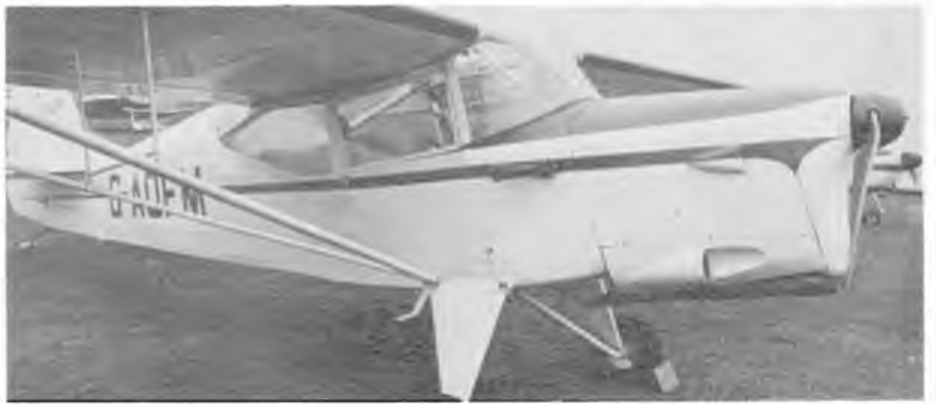
Above: plexi-glass cockpit glazing mouldings are complex on the Autocar (and expensive) the windshield fairings-in to the wing roots and over the wing upper centre section.
