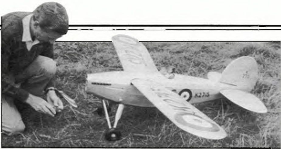
Above, Tony Turner is really hooked on Rupert Moore's 'Viper II' design. Two years ago he made the rubber powered original version, and now he has built a 'times two' R/C example with a beautiful laminated propeller.
