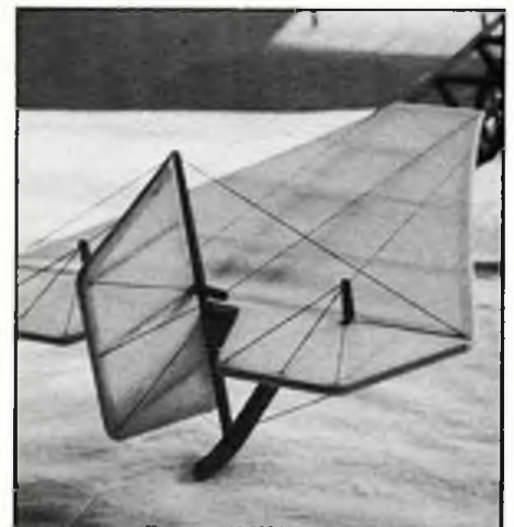
Above, how about this for a winter project... Martin Tuck's triplane is a real stunner in the air. Just make sure that your 'pole' is well secured to 'terra firma' before take-off. Below, detail of tail assembly shows simple structure enhanced by the addition of control horns and rigging 'wires'.
