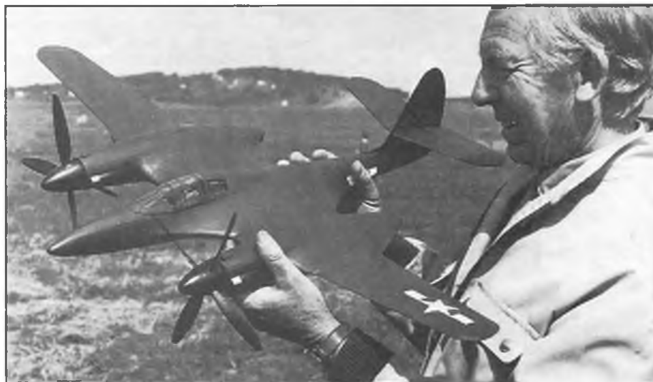
Above left: Lubomír Koutný, who supplied these inspirational photographs, holds his Arado Ar240. Model is built to 1/20 scale and is capable of over 70sec. Nacelles appear to be slightly longer than scale. Note fully-equipped cockpit. Above: Lubomír's son Peter with an exquisite Peanut Gloster VI, 1st place model in the Pardubice Seaplane Cup event. Above right: A nice pair - Lubomír's Ar240 and B1109F: winners both. Motive power for the Arado is seven grams of 6mm Pirelli, 600mm long (each motor).
