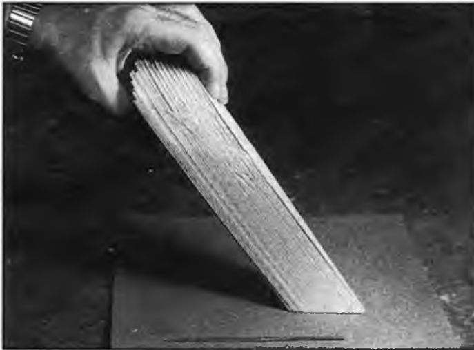
Note that the rib ends are carefully aligned here. Don't forget to align the rib sideways, and position the templates with centre lines parallel.
