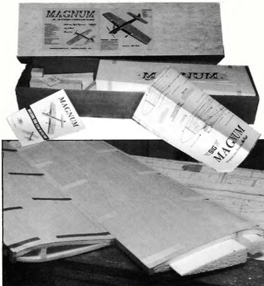
Open the box! Foam wings take up much space but there's lots more inside. Wood quality impressed our reviewer. Above: Wing tip and root of wing panels reveals hollow core. Panels have to be skinned by the builder.
