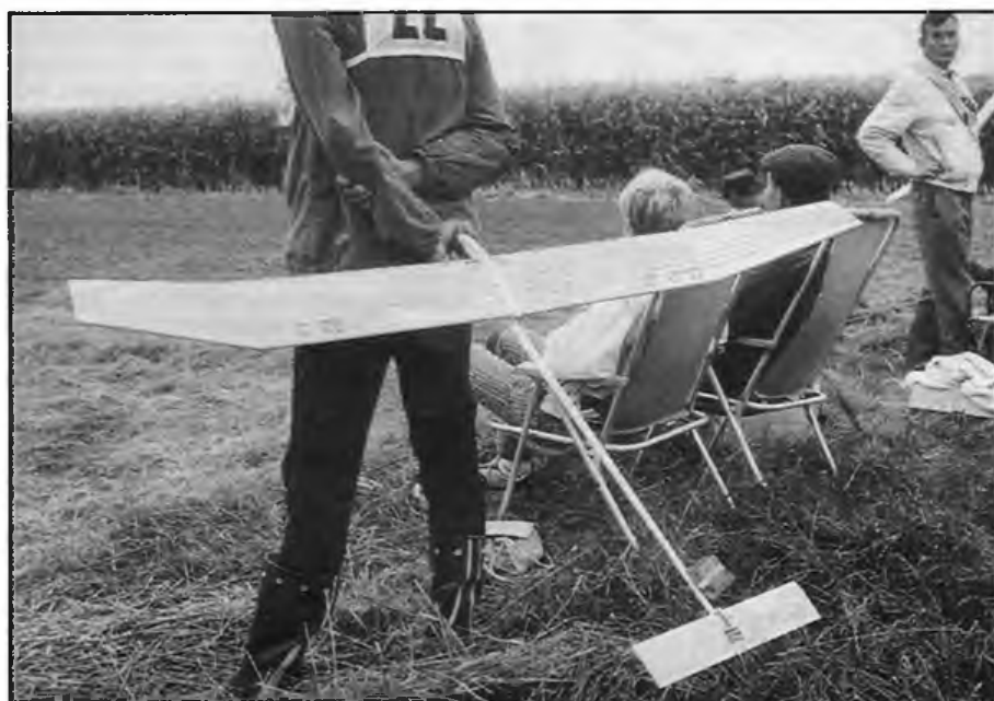
Winning F1A at the Eifel Pokal meeting. Crha's magnificently-constructed model features a foam wing, mylar covered.
