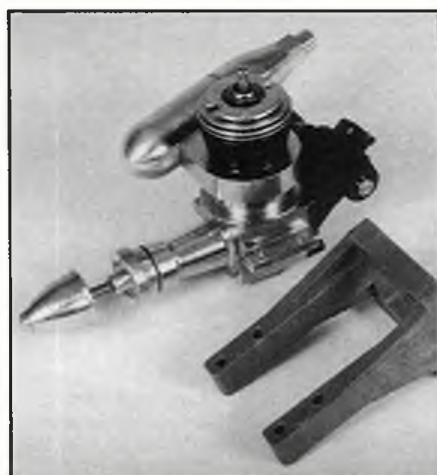
Cox Queen Bee .074 RC shown above and left, with purpose-built motor mount.
