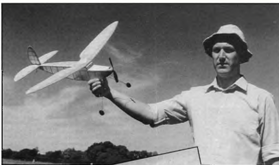
Above: Ted Gardener's Veronite No 1, 28 inches span, is electric-powered by a Derek Knight motor instead of rubber, as original. Left: Charlie Havis with his P E Norman designed Antspants. All-red model is fitted with wingtip slots and is replica Mills 1.3 powered. Foot of page: This double-sized Frog Interceptor, powered by a K&P electric motor, was flown by David Moul.
