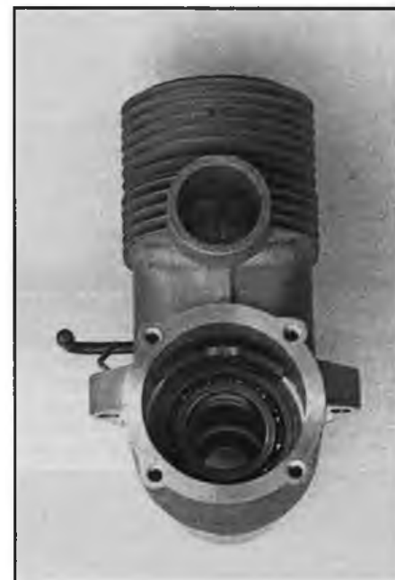
Rear bearing is housed in shrunk-in ring.
