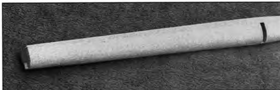
Leading edge features foam core, softened spars and wrap-around sheeting and balsa ribs, and is paper covered.
