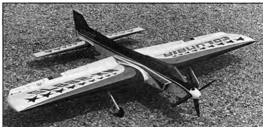
Jim Casale's (USA) stunter was the best finished of the lot. ST60 drives Bollenhagen four-blade prop.
