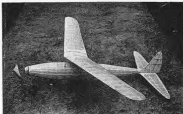
Another very interesting model. Note the single wheel and the high aspect ratio of the stabiliser.
