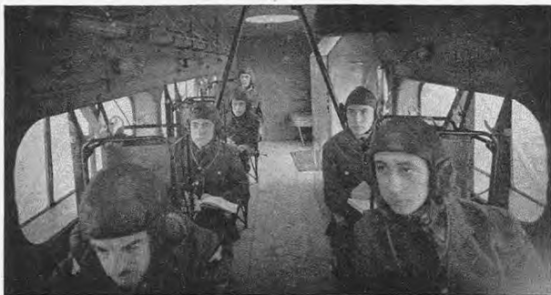
Wireless operators in a flying classroom. One of the two D.H. 86b's which is equipped for instruction in aircraft operation at Cranwell. There are two seats for instructors and six for pupils, each of whom has a receiver.
