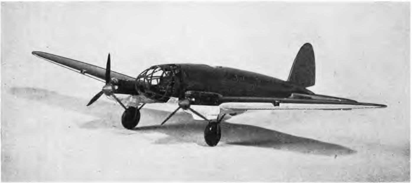
Fig. 4. A further stage in the construction. The nose-piece has been fitted, and there remains only the doors to the undercarriage and the gunner's windscreen to complete the assembly.
