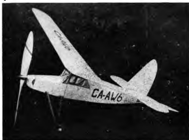
39 in. SPAN MILES TRAINER. 1 in. scale. Designed by J. H. Towner.
