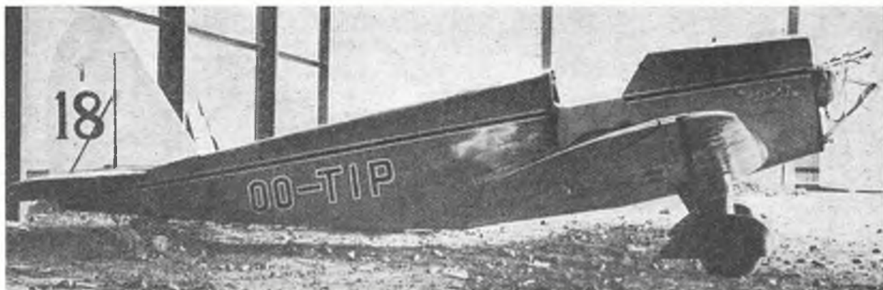
Right. The pronounced wing tip incidence wash-out can be seen in these two photographs of the Model B trainer.
