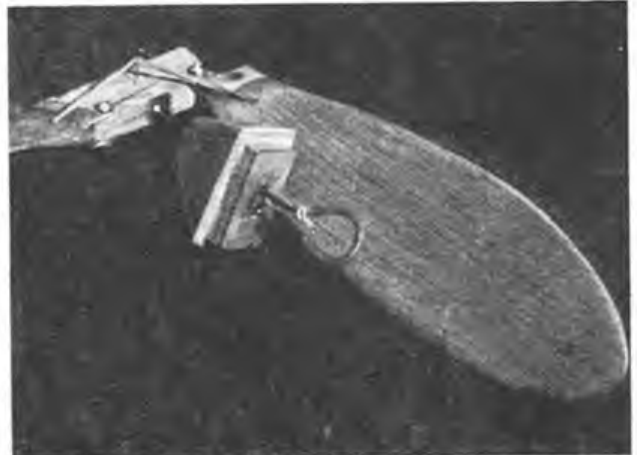
A folding airscrew assembly by Per Weishaupt of Denmark that weighs 1 1/2 ozs. Note the rubber tensioners on the blades for snap folding.
