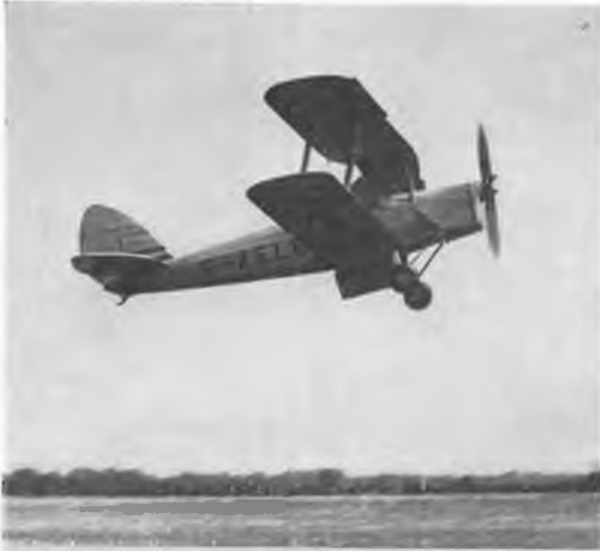
The model coming in to land. Note the nose-up attitude obtained with the automatic trimmer.
