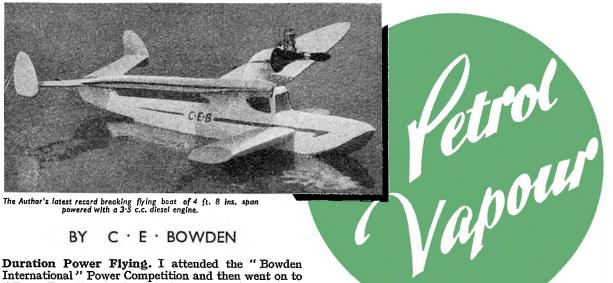
The Author's latest record breaking flying boat of 4 ft. 8 ins. span powered with a 3.5 c.c. diesel engine.
