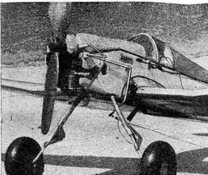
Fig. 5 (Above). A close-up of the Ignition control for engine-on landings, fitted to the author's Candy Mark I.
