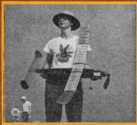
18. LEONARD DICKIE (28th) of Ottawa, Ontario, Canada. Flew a diamond fuselaged, parasol type model, parallel chord wing being sharply polyhedral. Twin finned and single blade folding prop. Had more than his share of troubles, and only crammed in poor flights in spite of sterling efforts. Times:—0 : 58.1, 0 : 55.2 and 0 : 11.8. Average:—0 : 41.7.
