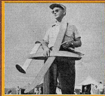
8. TOM CORYHILL (4th) of Indianapolis, Indiana, U.S.A. Top man in the American Wakefield team eliminator. Model was an "extreme" slabsider, with extra large cross section at rear end, presumably for rubber space. High wing with polyhedral tips, single wheel undercart and single bladed folding prop. Wide span tailplane with three fins. Times:—3 : 28, 7 : 37·2 and 1 : 42·8. Average:—4 : 16.
