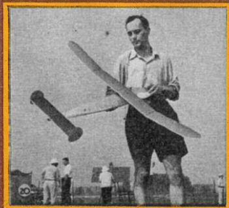
20. LUDO VAN HEMELRIJCK (9th) of Brussels, Belgium. Flew the standard Belgian model, employing diamond fuselage, and all sheet balsa covered high aspect ratio wing mounted in parasol position. Wings were braced with thread, and looked generally unsafe even in calm conditions prevailing at Akron. Not much chance in average English weather. Times:—1 : 03.4, 7 : 00.9 and 0 : 13.4. Average:—2 : 45.9.
