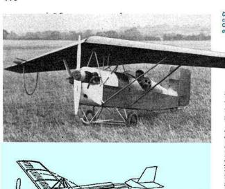
On the left: The Granger Bros<sup>\*</sup> Tailless Aeroplane designed and built by them and completed after four years work in 1930. Powered by 30 h.p. Bris'ol Cherub. On the right The tailless aeroplane in flight near Tailerton An amazing amateur achievement, built for the most bort in a garage assisted by simply model both.
