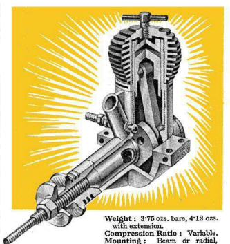
upright or inverted. Recommended Airscrews: Depends on type of model. Tank: Not fitted. Bore: '6875 in. Stroke: '5625 in. Cylinder: S.14, hardened, ground, honed, round and parallel to 00005 in. 10 ports; 5 transfer, 5 exhaust. Screws into crankcase.
