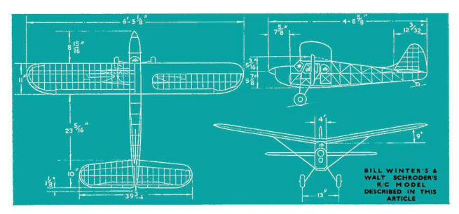
flying in all conditions, we eventually returned to the 14-inch propeller, flying the machine at higher speeds and compensating fore-and-aft trim with increased downthrust. This brings up one of our first real lessons, which is that it is best to design a machine with a minimum difference between power-on and power-off trim, hence minimum down thrust. This is possible by keeping the thrust line close to the wing, as exemplified by the Good's Rudderbug.
