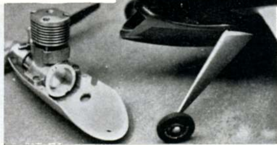
Detail of Bernard's light alloy mounting pan for the Oliver Tiger Mk. 3 and Edmond's type rectangular tank mounted diagonally for gravity feed
