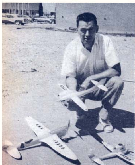
United States National Champion for 1957 was Jim Payson. He is holding his very special "65" engine sidewinder speed model, with engine blown up from Fox 39R to larger capacity. Proto speed model with a Fox 29X is on ground at left, and his Class B speed entry with Fox 29R which set a record at the Dallas Nats is at right. Jim obviously goes for swept fins!
