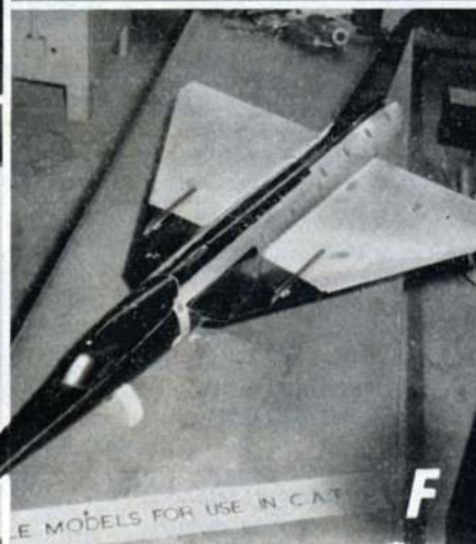
(A) Friendship by ace Polish modellers, Datkiewicz and Nachtman, shows interior detail. (B) Saro have their own modellers for SRN.1, as do Blackburns with their product, the NA 39 in (C). Picture (D) shows Airco DH 121 by Master-models to one-twelfth scale. (E) is a DC-8 by same firm, Laurie Barr, Managing Director, checks finish on huge 15-ft. span model. (F) is the mixed metal/wood FD-2 used at N.P.L. for compressed air tunnel research
