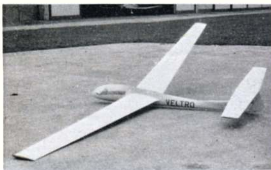
Russian power gimmicks for fuel feed and slip-stream control, below. Right, J. Nicoud of Lausanne designed elegant 126-inch glider. Has 1 c.c. power pylon for calm, detachable tips for wind
