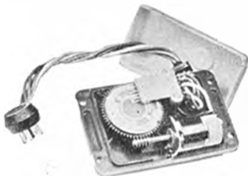
The "works" of the Unimatic servo, seen with case bottom removed, shows p.c. disc and wiper bank imposed and worm drive from Microperm motor
