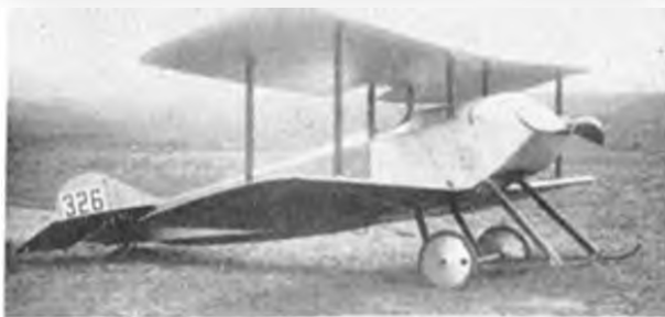
Aircraft 326 with warping wings and landing skids. I.W.M. photo MH3286 Naval seaplane 3804 on twin floats, showing increased fin area. I.W.M. photo Q67584 Bottom, racing No. 14 on Tabloid with Vee strut undercarriage, showing cowl intakes. Flight photo 0195
