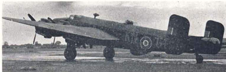
B.Mk.III of 77 Squadron R.A.F. (oddly enough the 'Lancaster Squadron') at dispersal showing the H 2 S radar bulge, tapered tips of enlarged span and 'weathered' colour scheme.
