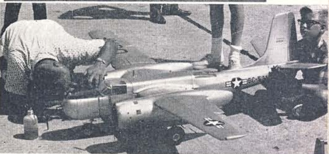
Above, B-26B control-liner by Edward Shea of Columbus, Ohio. Span is 7 ft., weight is 18 lbs. Powered by two Super Tigre .50's, obviously takes some holding.
