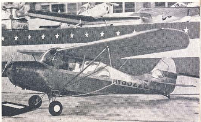
Below: 1947 Aeronca 7AC Crop Sprayer by Richard Hansen of Cozad, Nebraska. Everything works including the spray rig! Span 77 in., power by Fox 74, Logitrol equipment.
