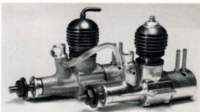
Left, the 1954 diesel and 1955 glow model McCoy 049 cylinder assemblies. Note O-ring equipped contra piston and unusual glowhead arrangement. Despite outward similarities, engines used different crankcases, shafts, pistons and con-rods as well as different cylinder assemblies. Above, two vintage McCoy 049's. These were introduced in 1954 and 1955. The long intakes each housed a clapper valve between the jet and rotary-valve - a unique arrangement.
