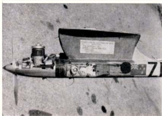
12. 'Night Train' complete with Miebach, pipe and Seelig timer used by R. N. Hewitson of New Zealand, proxy flown by Jack Allen.
