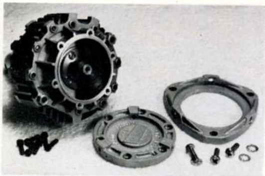
Rear view of engine, less cooling ring, with radial mount and rear cover removed to show rear counter balance.
