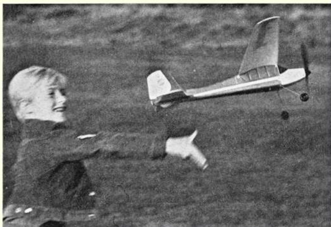
Left: Airborne and climbing fast, SuperStar accelerates rapidly as the coarse pitch 7\frac{1}{2} in. diameter propeller takes hold. Above, Jonathan releases into a left turn, the best natural flight pattern to cope with high torque. Wing has ready-formed airfoil camber and required no adjustment of incidence angle.
