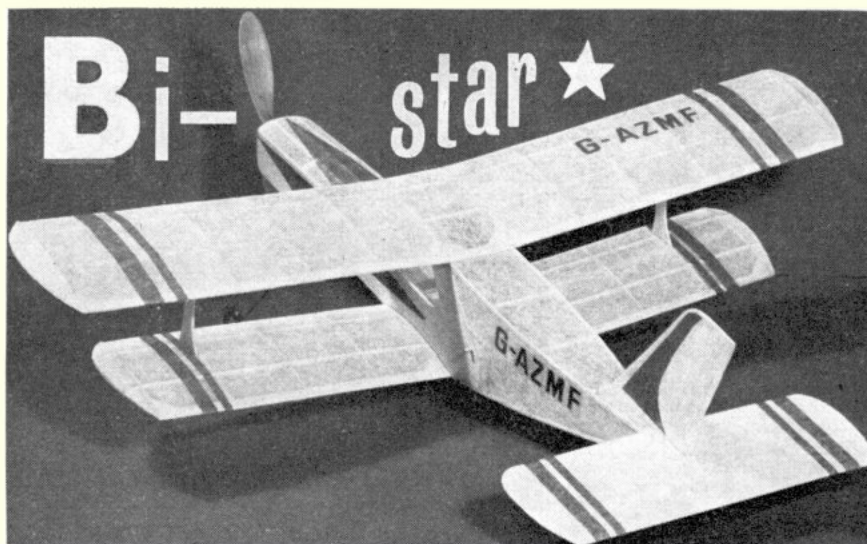
Delightful 18 in. span rubber-powered sportster designed by RAY MALMSTROM
