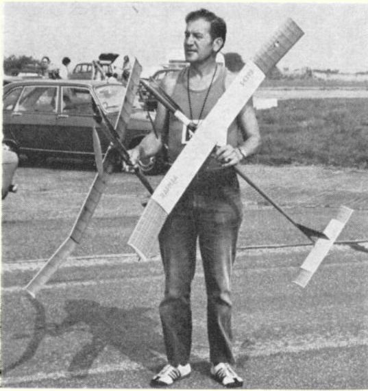
'Butch' Hadland, representing the Royal Air Force Model Aircraft Association at FFN International Contest, Strubby, with his pair of Wakefields which have curled down tips to improve airflow.
