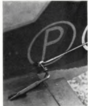
Close up of the flap linkage reveals pushrod from the bellcrank passing through the flap horns and the fuselage itself. A second pushrod then provides the connection to the elevators.
