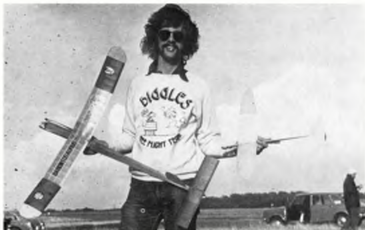
Left: Martyn Cowley had a successful day out at the Southern Gala with two third places with these designs. The Coupe d'Hiver model is eight years old and features turbulated propeller blades and Montreal stop, while the chuck glider is of rather more recent vintage, incorporating a high ridge point airfoil and swinging weight D/T. Picture on opposite page shows John Barton who took second place at the South Bristol Gala in the Vintage Precision event. He flew the Norman-Marcus designed 'Bazooka' that won the last Hullavington Nats. Model uses a tip-down tail D/T.
