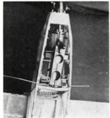
Underside of the Keil Kraft Competitor shows the Monogram E-Power unit fitted - and the access hole necessary for connection of the re-charging battery. This unit is best suited to a 'permanent' installation rather than to attempt making it interchangeable with other models.
