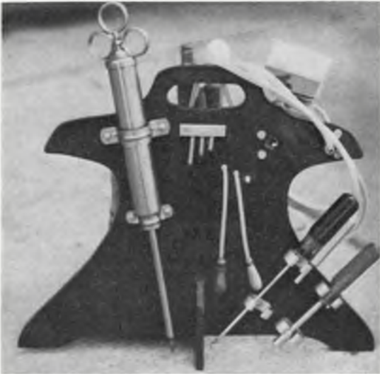
Two views of Bill Allen's (USA) 'Combat Pak' - which eliminates 90 per cent of the problem in a pit stop. A 2 volt battery with a special buzzer system and ammeter check and double check for 'dead' or flooded plugs. Light and handy, it carries everything needed in an emergency.
