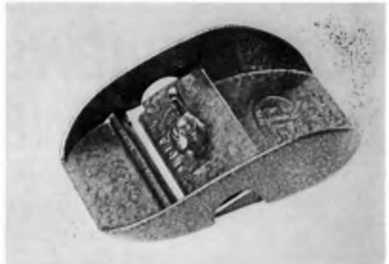
One of the best 'tips' of all is to purchase a razor blade plane, such as this 'Zip' plane. Using razor blades as the cutting edge, it is an essential part of any modeller's workshop - being perfect for shaping solid balsa wings, leading edges etc.
