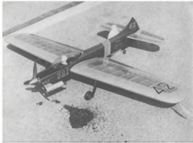
Winner at the Bochum International was Dr Egervary flying this very functional design with Veco 50 power. No cowl is employed but the wings are detachable.
