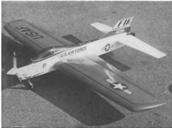
An F-16 inspired stunter is the latest from Yves Fernandez, using the same wing and undercarriage as the Scirocco. A Czech muffler weighing just 15 grammes is bolted to the ST46.
