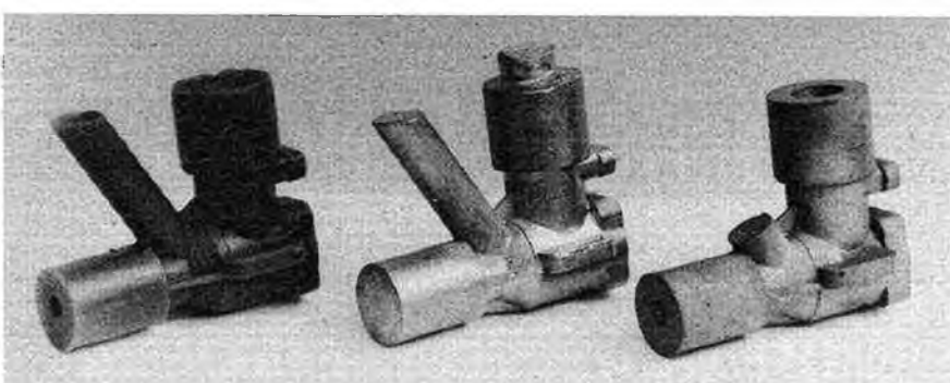
Evolution of an investment cast crankcase. Left to right: (a) wax pattern; (b) solid crankcase as cast in LM4 aluminium and (c) rough machined and heat-treated unit ready for final machining.
