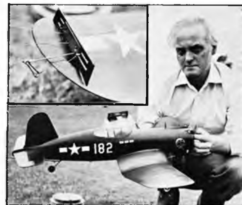
Brian Young's winner of the Profile 40 event. Model incorporates flaps and kick rudder. Peter O'Sullivan with his Irvine 40 powered Corsair. Inset: detail of Peter's adjustable line outlet on his Corsair.
