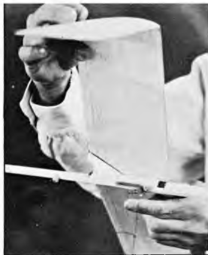
Mick Page with his folding wing HLG which is based on an American design by Stan Stoys. Detail of Mick Page's folder. The wing is held in place by a hook, which in turn holds the wing folded through the launch by means of an air pressure vane. Theoretically this releases the wings at the top of the launch.
