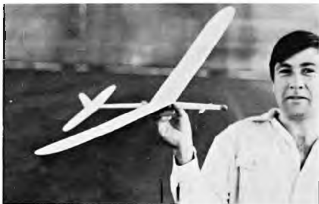
Mick Page with his folding wing HLG which is based on an American design by Stan Stoys. Detail of Mick Page's folder. The wing is held in place by a hook, which in turn holds the wing folded through the launch by means of an air pressure vane. Theoretically this releases the wings at the top of the launch.
