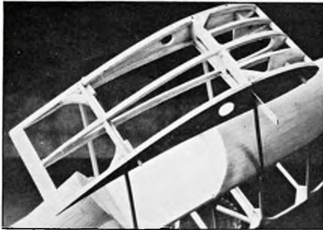
Wing centre section and cabane structure. Before gluing the centre section to the cabane struts, ensure that you have the correct angle of incidence and the wing is square to the fuselage and tailplane assembly.
