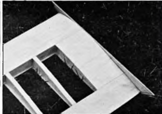
With the end plates fitted, join wings and mount on the fuselage. Shape soft balsa block to fair wing into fuselage form.
