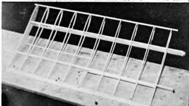
Right: wing ribs and laminated ribs. In the foreground, polystyrene former for laminating the 1/32nd tips around. Left: pin the trailing edge down on the building board while gluing ribs and ensure leading edge is parallel to the trailing edge.
