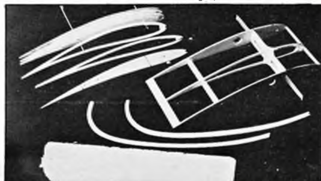
Right: wing ribs and laminated ribs. In the foreground, polystyrene former for laminating the 1/32nd tips around. Left: pin the trailing edge down on the building board while gluing ribs and ensure leading edge is parallel to the trailing edge.
