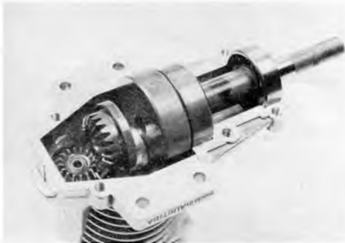
Below left: vertical drive shaft is geared up, through bevel gears, to run at 1.25 x crankshaft speed 2.5:1 spur gears at top reduce rotary valve to required half crankshaft speed. Right: carburettor, shown dismantled, is two-needle, automatic mixture type. Black finished exhaust stub and silencer are made in one piece.
