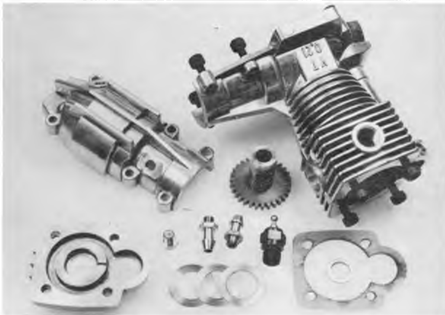
Engine's main casting includes integral cylinder head. Also shown here are crankcase bottom, rotary valve and spur gear, head cover, valve shims, pressure nipples and glow plug
