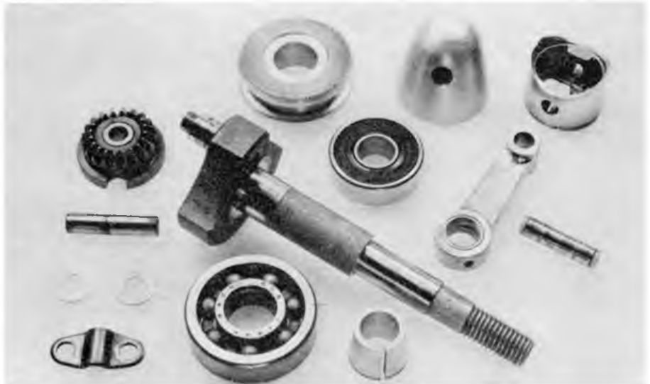
Other parts of VT-21. Note sturdy crankshaft, slipper piston and short conrod. 'VT' stands for Viertakt, the German for four-stroke
