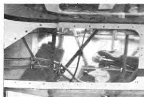
Left: tail brace and control-link detail; at right, clear panels afford illumination to the cockpit area. Below left: large span ailerons are readily apparent while, below, a well-braced tail unit. Below right: the distinctive NACA duct on the rear fuselage. Photos: A. A. P. Lloyd.
