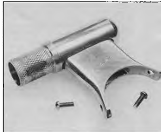
Above left: Dunham Orwick crankcase and contact breaker parts: case is stove enamelled green like original. Below left; minor modifications to Dunham Orwick include transfer windows in piston and cylinder and slightly modified combustion chamber. Below; special Dunham exhaust duct with right-angled outlet to facilitate fitting silencer to Orwick Replica.
