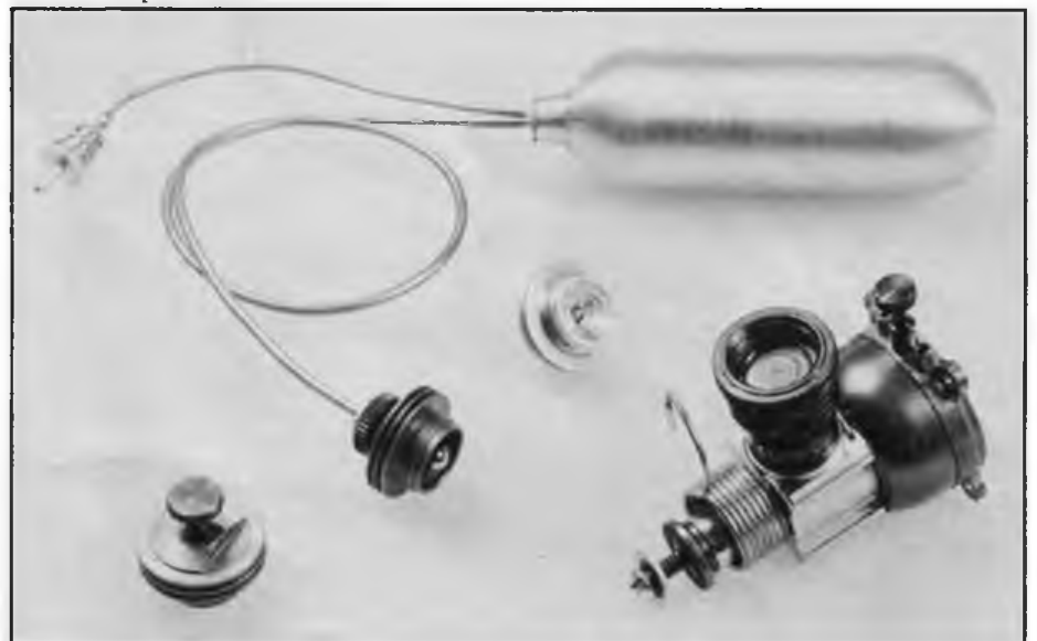
Left: unique CO 2 conversion of Cox Pee-Wee 020 is by diesel conversion specialist Bob Davis. Below: basic Pee-Wee 020 with its glow head removed (centre) and showing alternative Davis diesel head and CO 2 conversion.
