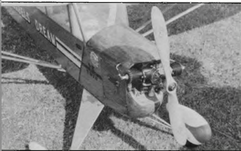
Left., Close-up of the O.K. Twin in Jim Shelley's 'Mable's Dream' (see text) A weak point of this engine lay in the crankshaft, but Jim has already modified this component to provide a reliable unusual vintage power plant.
