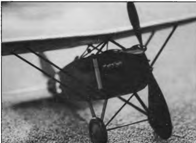
Left., the radiator on the fuselage side is a prominent feature of the "Gosling".
