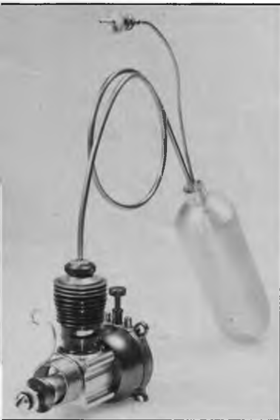
Left: unique CO 2 conversion of Cox Pee-Wee 020 is by diesel conversion specialist Bob Davis. Below: basic Pee-Wee 020 with its glow head removed (centre) and showing alternative Davis diesel head and CO 2 conversion.
