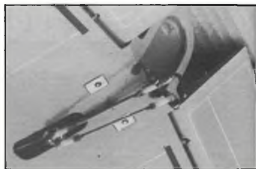
Above, painstaking attention to detail is the hallmark of aircraft built by Franco Ballesio, as this picture of his swept-forward 'Astro' shows... Below, as the flaps are not in line a twin yoke control system is required.
