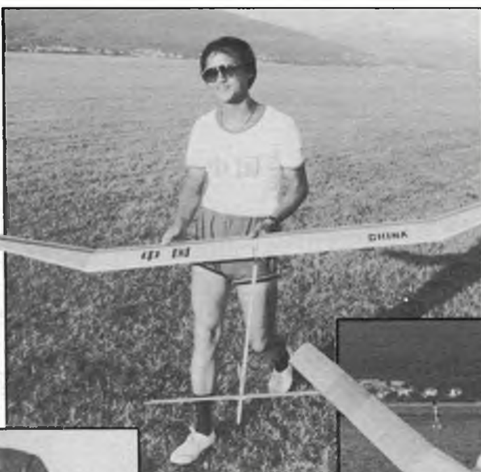
Left, Yue Liang's winning model is constructed from Chinese Tung wood with sheeted D-Box and carbon fibre spar caps. Yue has developed a unique pendulum latch tow hook, which prevents accidental release.
