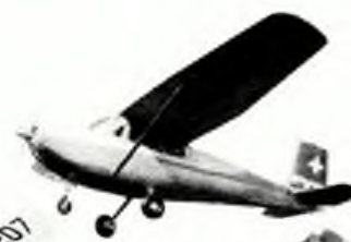
CESSNA 172 By W. P. Holland. This 72 in. (1829mm) 1/6th scale model of the popular American light-plane is the answer to those who want an easy-to-build large model for radio conversion. Knock-off wings and shock absorbing trike u/c. For 2.5-3.5 cc engines. FSP/668 Price £4.40
