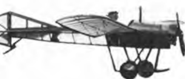
SUPERMARINE SPARROW by G. F. Elsegood. 1/12th scale of 1920's light racing aircraft designed by R. J. Mitchell; 34 in. (864mm) span model features scale rib spacing and pendulum rudder/aileron controls. For 0.3-0.5 cc motors. FSP/1408 Price £1.80
