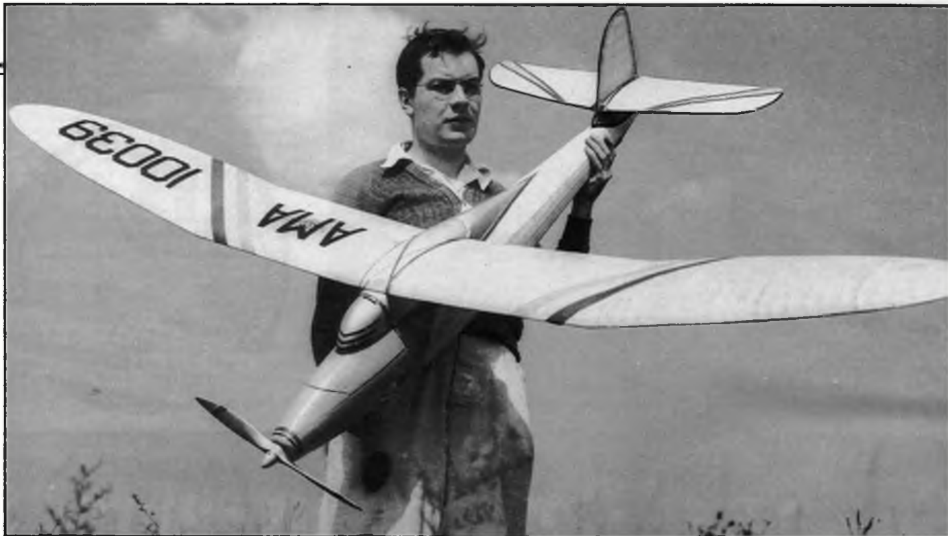
Tom Perzentka with the 72in. Ott Streamliner with monowheel undercarriage. Power was supplied by an inverted - and buried - Dennyrite Airstream which drove the propeller through a five-inch extension shaft.
