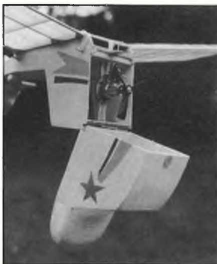
...but Starstream is equally happy with Cox Pee Wee 020 power - as shown on the plan - although a three-bladed prop will be needed.
