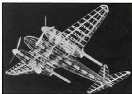
Above: The Ott-O-Tube Mosquito featured moveable control surfaces and retractable landing gear. Below: The prefabricated 58in. R/C Golden Falcon which Joe Ott designed and engineered when he was over eighty years old.
