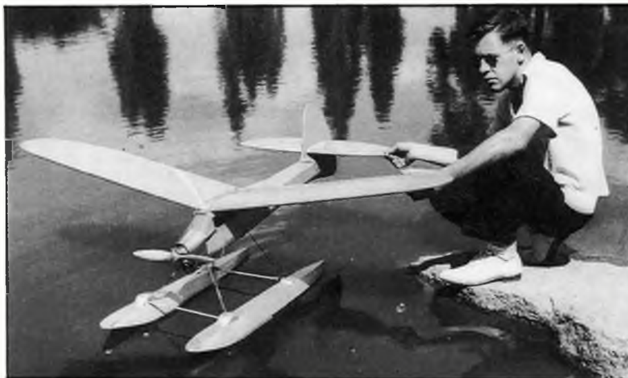
Walter Fromm seen in August 1939 with one of four development models of the Kingfisher; here it is seaplane guise with Joe Ott designed 35in. Silver Flash Pontoons. A change to wheeled landing gear was claimed possible in only thirty seconds!
