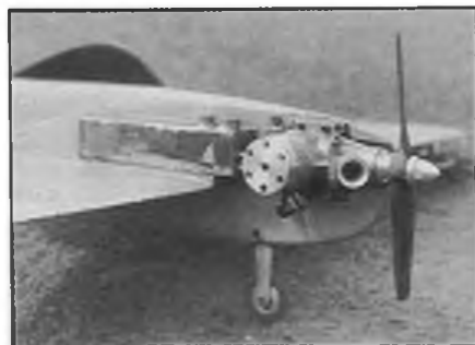
Self-venting tank valve, double tube crusher shut-off and adjust-by-key needle valve all visible here.
