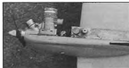
Outer edge of tank is just outboard of the needle valve. Shut-off button, here re-set, is in minimum drag position and falls naturally for refuelling.
