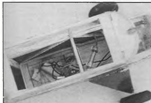
Above: Nose details of the Sheppard sportster. Four 150mAh cells used. Special wide-blade prop here removed; comes with motor unit though. Left: Plenty of room for wiring and fuse.
