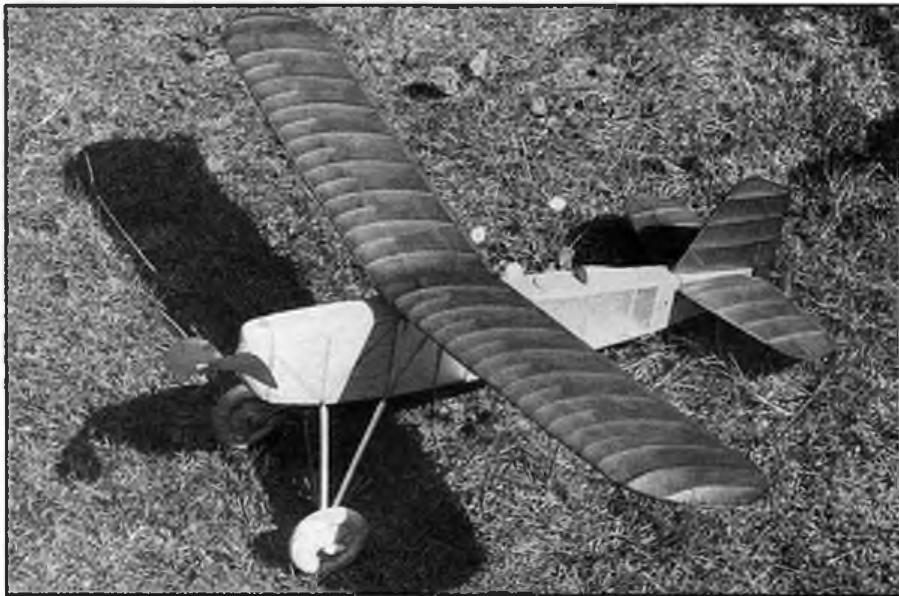
Nondescript Bluebird. Blotchy 'camouflage' finish was due to tissue dye and dope interaction.
