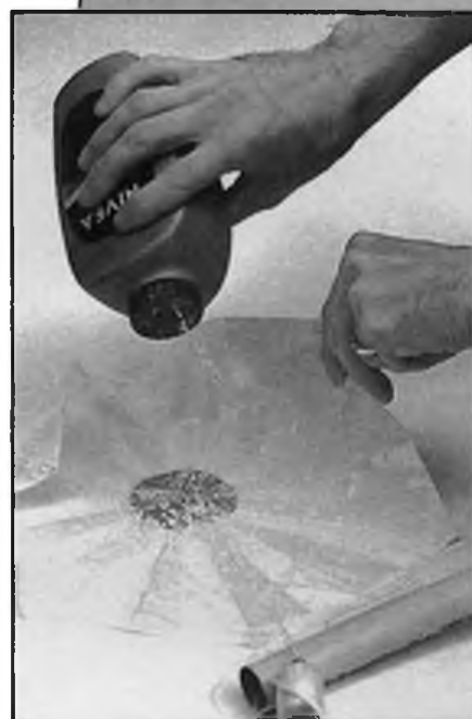
Static electricity builds up fast in the plastic parachute during flight but talc or flour ensures deployment.
