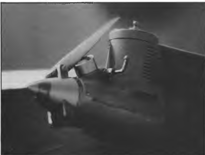
Left: Interesting purpose-built F1C motor by Leonid Fuzeev, seen at the Kiev World Cup event, features three-point radial mount and built-in brake.
