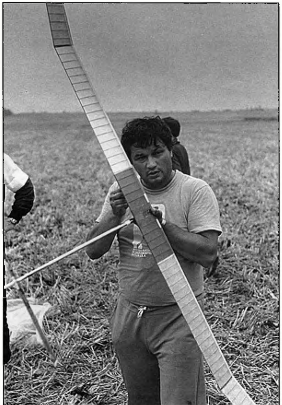
The incredible Stamov just prior to a series of flyoffs against Rump; wing appears to be tissue covered with much carbon structure, including solid carbon trailing edge of very small dimensions.
