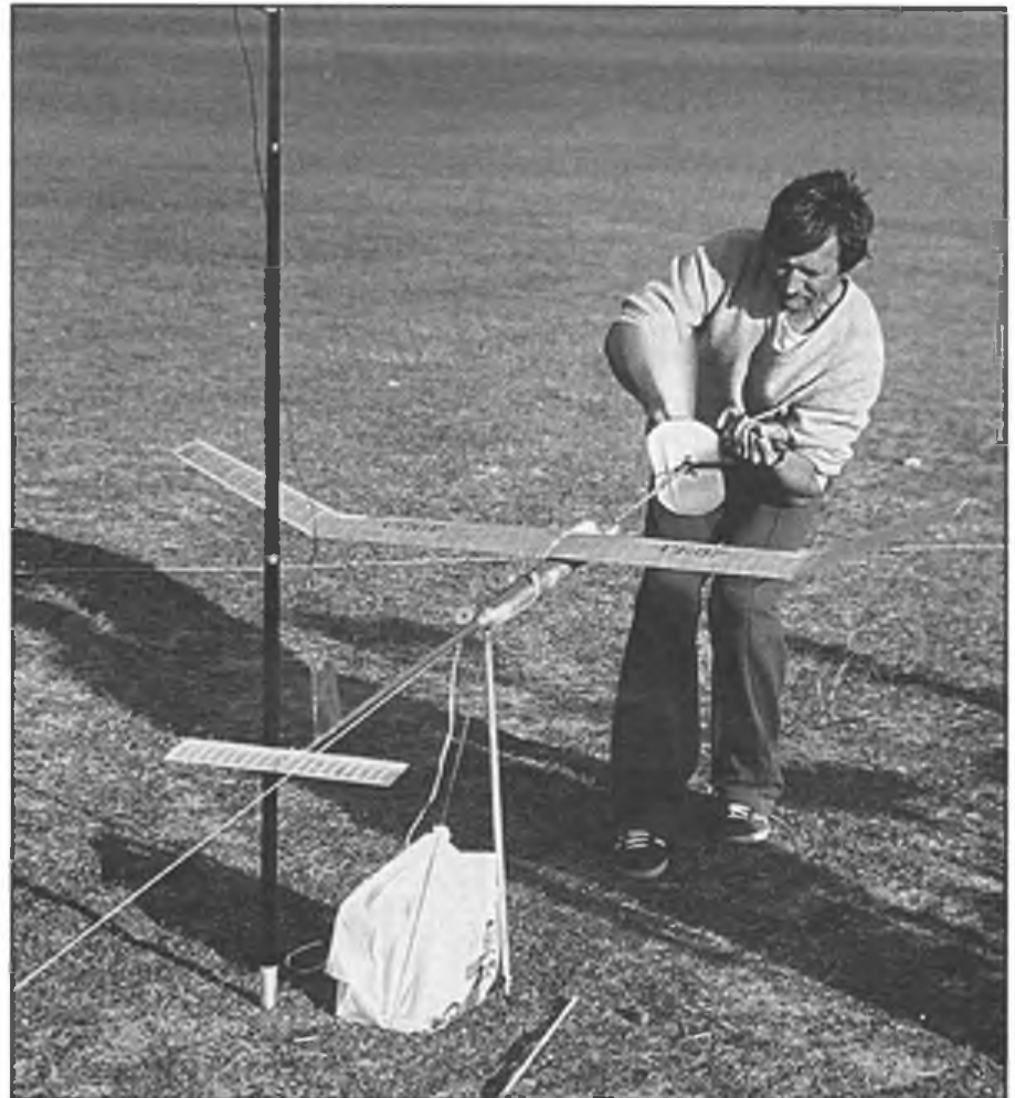
The Russian Gorban puts everything into winding for the penultimate F1B flyoff round at Domsod; broke two motors but eventually got away well. Note wires leading from heating jacket around motor tube to battery under winding jig.
