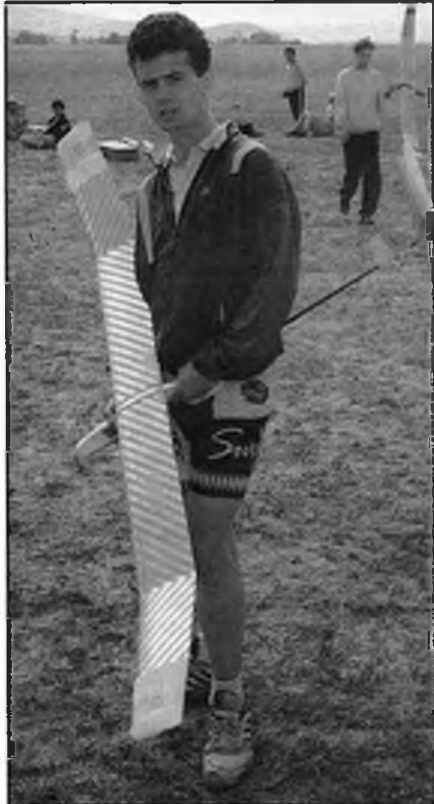
Anthony Ball with straight-tow-foam-and-paper-surfaced F1A model.
