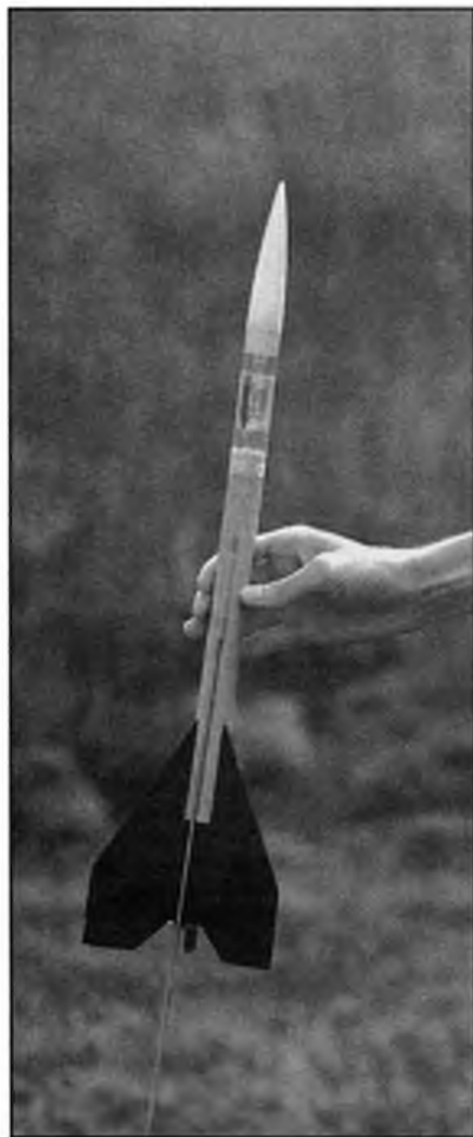
Hercules being mounted on the launchpad. It is important to lay off the angle of ascent to allow for wind.
