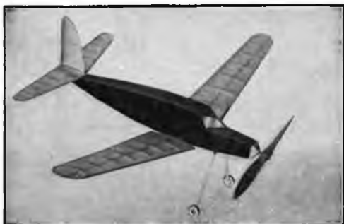
Span 29 in. Overall Length 18½ in. Total Weight 1½ oz.
