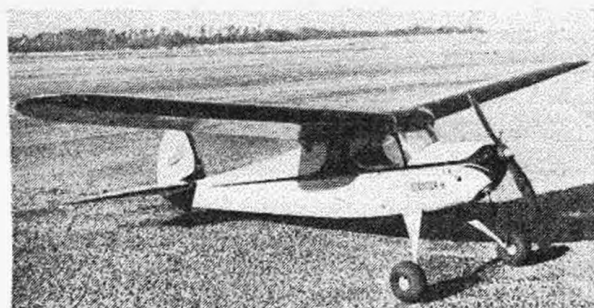
Photo 4. The 23" span diesel model fitted with "full-length slots by the author and powered by a 1½ oz. "Majesco Mite" diesel.
