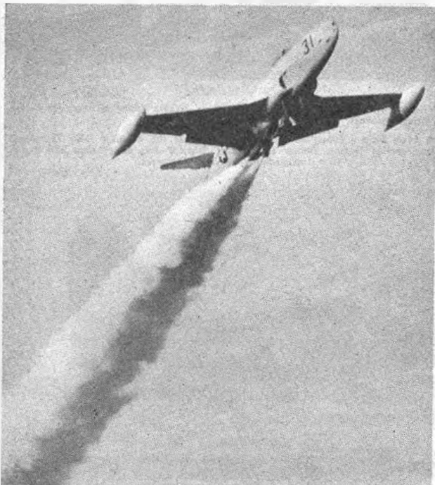
A P-80 climbing rapidly after a rocket-assisted take-off. The clean lines of the P-80 may be gathered from the photograph above.
