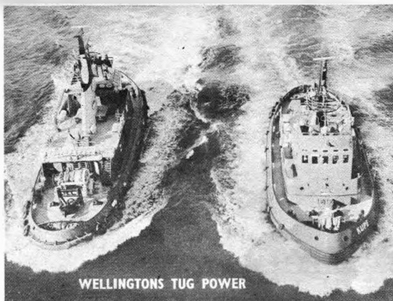
'Toia' and 'Kupe' demonstrate their prowess — one ahead, one astern at twelve knots! Incredible manoeuvrability is result of oscillatory propulsion unit. Photo: Wellington Harbour Board.
