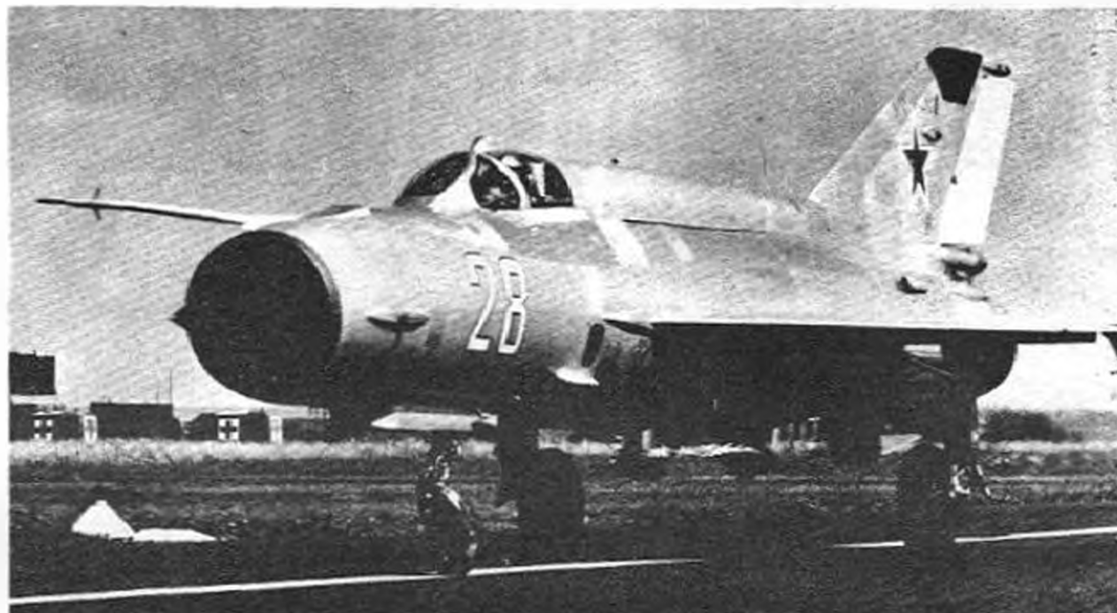
One of the MiG-21MF ('Fishbed J') aircraft which visited Rheims in September 1971. This version has provision for two 23-mm short-barrel 23-mm cannon under the fuselage between the nosewheel and the ventral pylon. (In the photographs, they are below the suction-relief doors ahead of the wing.) Also note-worthy are the rear-view mirror and the deepened dorsal fairing aft of the cockpit. (Photo: SIRPA-Air, Paris, France, ref. 33184).
