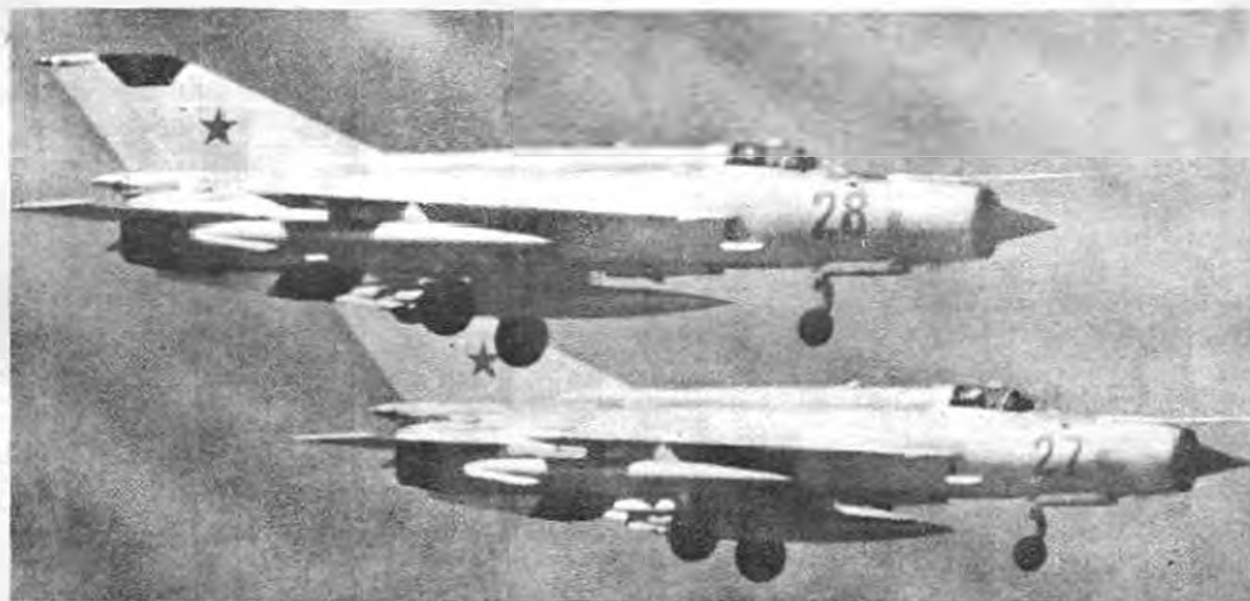
Two of the six MiG-23MF ('Fishbed J') aircraft which visited Rheims, France in September 1971. This model has two short-barrel 23-mm cannon between nosewheel and ventral pylon. Note the three underwing and fuselage long-range fuel tanks. Photo: SIRPA-Air, Paris, France.
