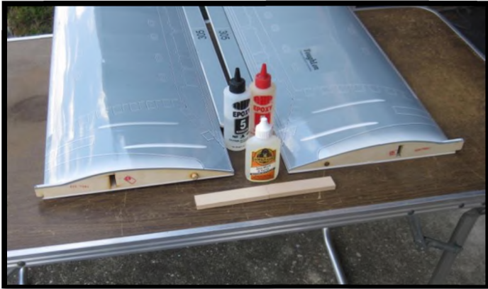
This photo shows the wing panels, the hardwood joiner and the two glues, Gorilla and 5-minute epoxy.
