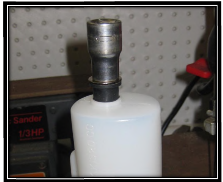
The 1/2" socket in place to put pressure on the plug assembly to force it into the tank. The socket is long enough to clear the feed and pressure tubes, allowing you to press the hard rubber plug in place.
