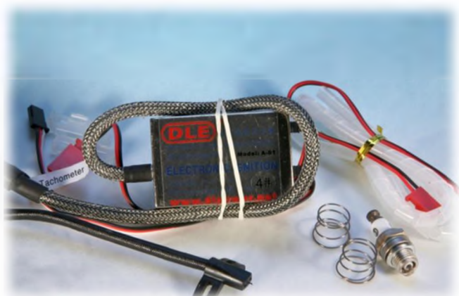
Ignition unit and supplied items. Note the 4# label.
