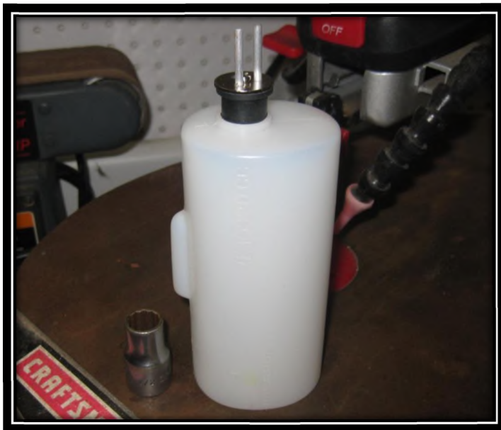
The tank plug assembly on top of the tank with a Craftsman 1/2" socket.
