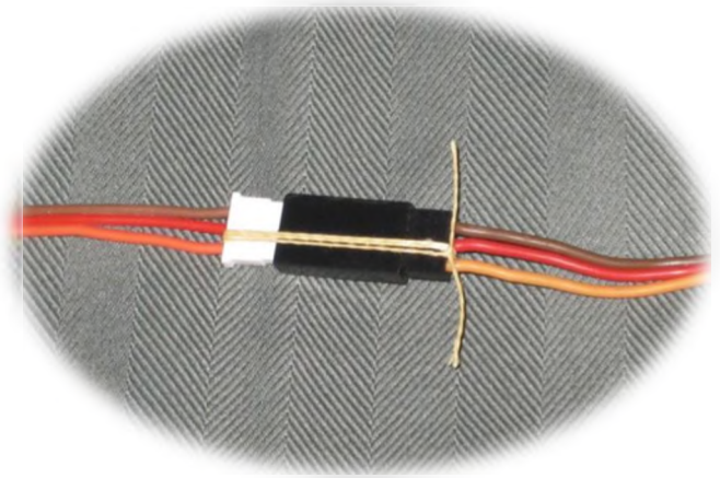
Shown here: the extension tied on to the servo lead with 30-pound test, Kevlar fishing line. Any string will work as long as they can't be easily pulled apart.
