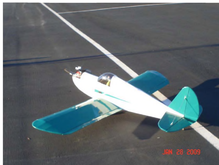
Photo2: Here's another of Frank Tanforan's planes. This one is a Doc Matthews' design that Frank scratch built from plans. The power is a Saito 150. He says it makes him look good.
