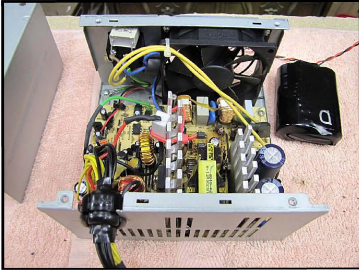
Photo 6: Here's what the PC supply looks like after most of those wires are removed.
