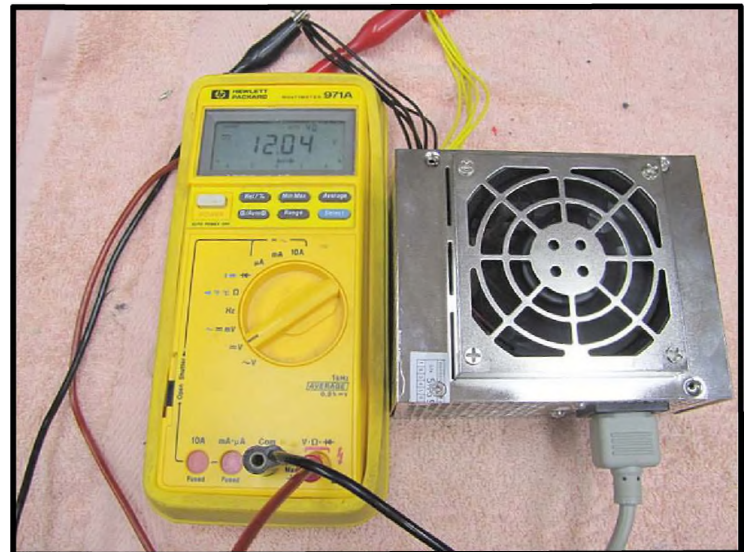
Photo 7: Look at the meter. 12 volts is exactly what we were looking for
