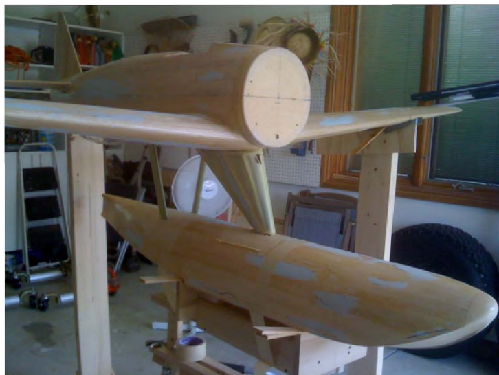
Photo 7: The main float, strut, and V struts all in alignment on the jig with the fuse and wing, ready for permanent attachment. Note tape holding float in place along with wooden shims to help in the alignment process.
