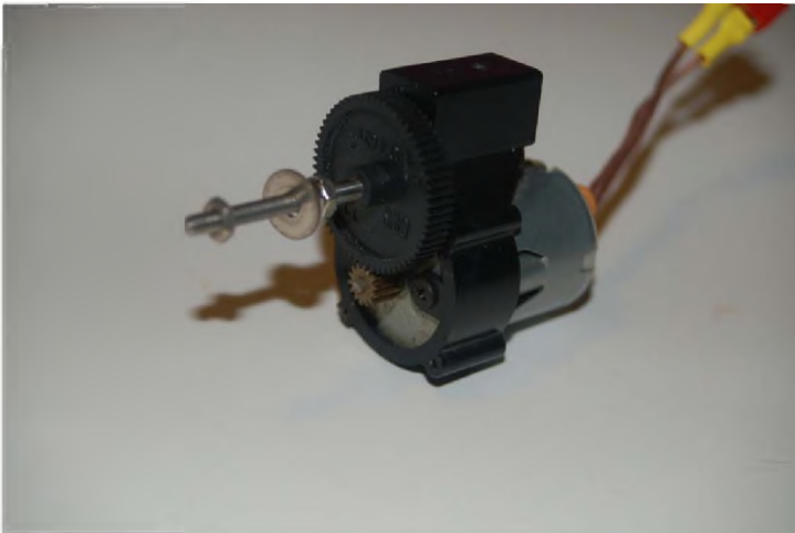
Photo 3: This is one of the very popular gear drive units that made GWS foam airplanes a big hit. Without them, the small brushed motors just wouldn't have the clout to pull most park flyers through the air.
