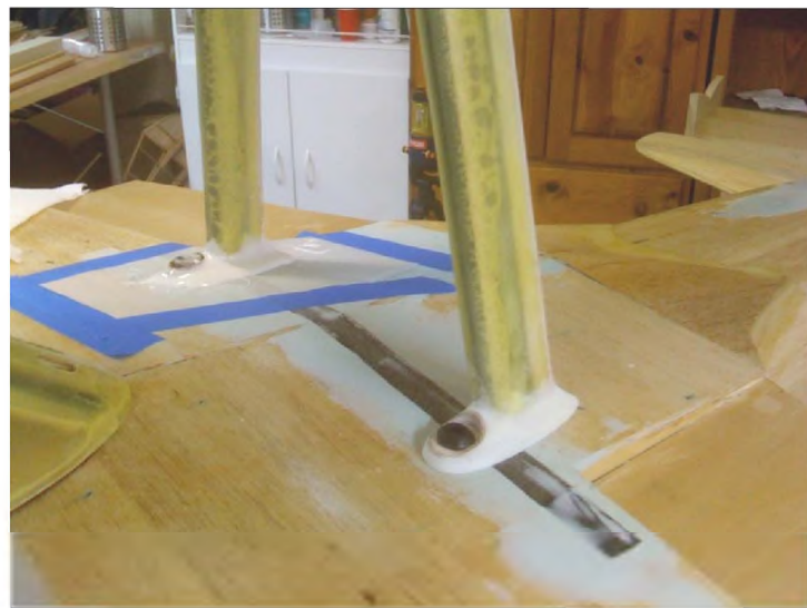
Photo 8: Here we see the way the top of the V struts are made. First ply plates are attached to the struts and then micro balloons and epoxy mix added to give shape. Note plastic sheet between strut and bottom of wing to act as a parting agent, and the carbon fiber tape glued into the bottom of wing along the rear spar for added strength.
