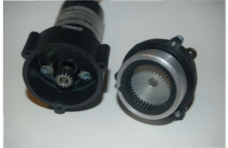
Photo 4: This disassembled inner-driven gearbox shows how the gears interact. They are much like standard pinion/spur drives but the output shaft spins in the same direction as the motor.
