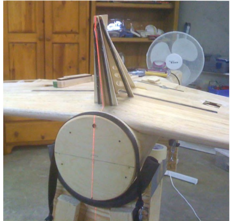
Photo 3: A Laser being use to align the main strut to the bottom of wing. This allows Robert to get the shape of the top of the formers to match the wing dihedral before top plate is installed to it.
