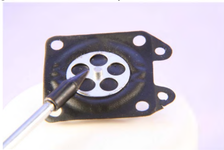
Photo 10: The pointer indicates the small extension on the diaphragm that activates the needle arm.
