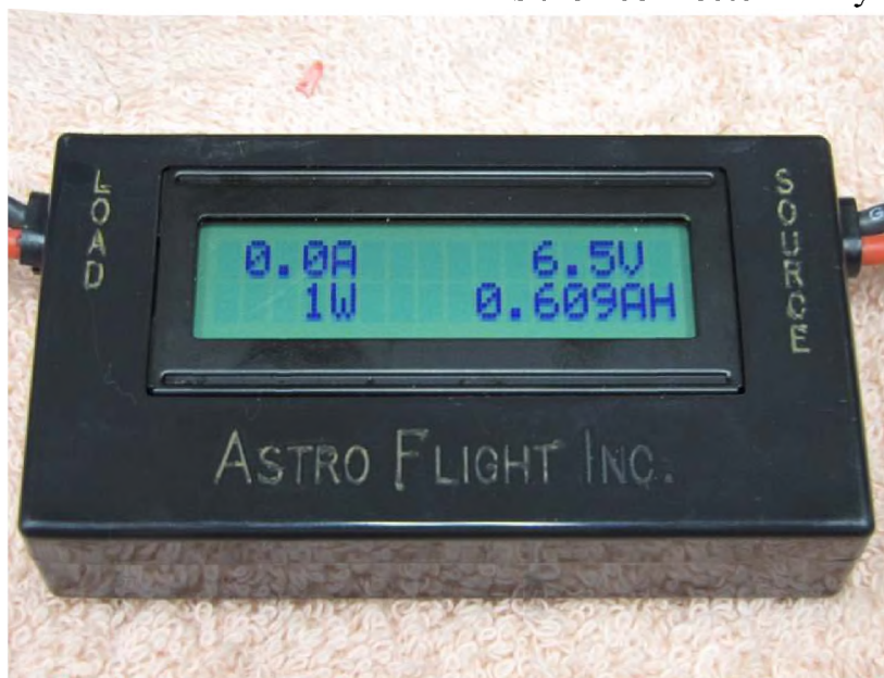
Photo 2: The Super Whatt Meter from Astro Flight used to measure charge replaced.
