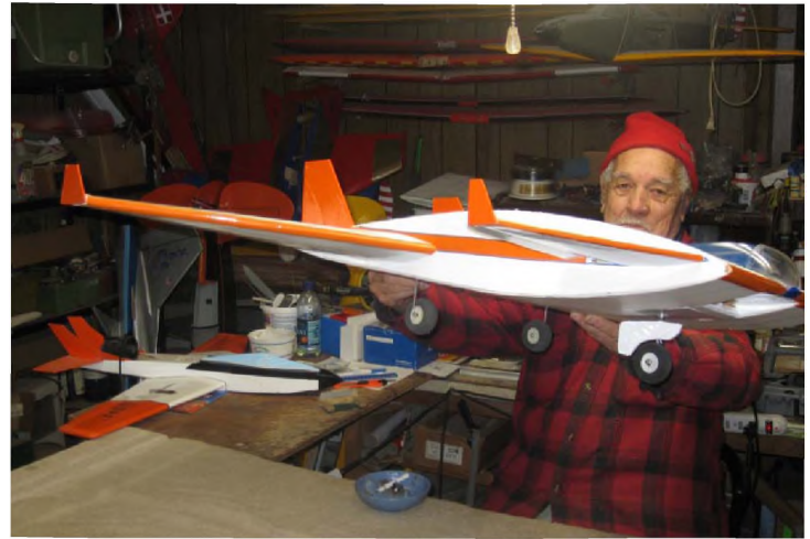
Photo6: Another view of Flaps and his modern Burnelli jet design. Note that the fuselage is a big, thick airfoil. Don't ask where the CG goes. We're going to wing it! I'll keep you advised on the testing.
