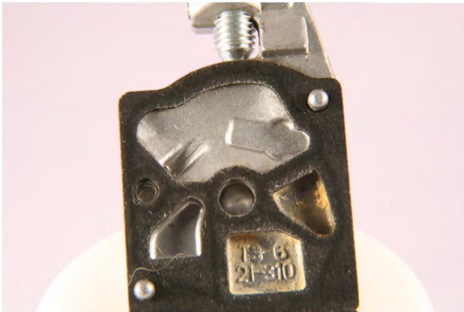
Photo 7: Gaskets and the diaphragm are keyed in place by opposed pegs.
