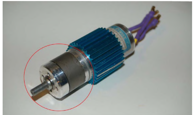
Photo 5: The planetary drive (circled) on this brushless motor can handle a lot of power and will fit in a small space. They're often used in high-performance gliders.
