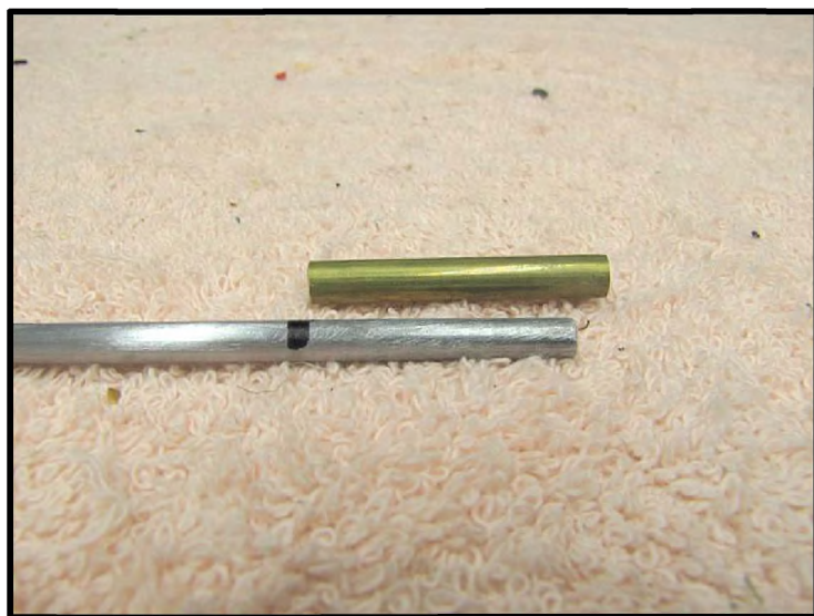
Photo 8: Brass tubing and music wire axle used to mount vintage wheels.
