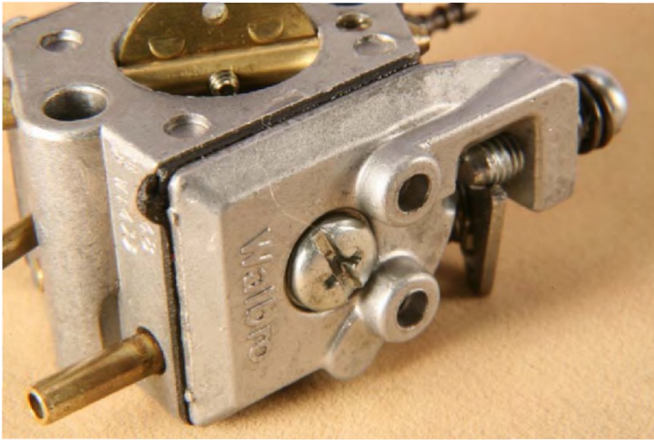
Photo 5: This is the cover you remove for access to the filter.
