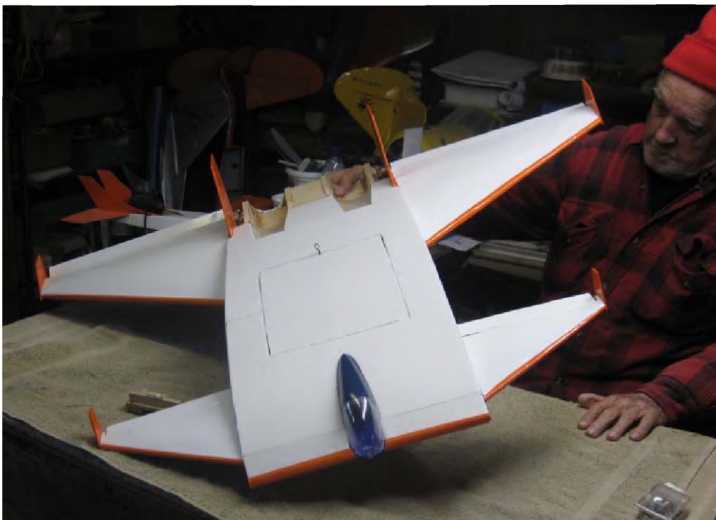
Photo5: Flaps' new creation has no name yet. You might remember the CBY-3 Burnelli, lifting fuselage design he built and I flew. He found an artist's drawing of a modern Burnelli design with jet power that he liked. To top it off, it was a canard! He just had to build it. The electric ducted fans were on order when this was written.
