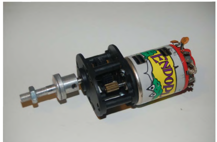
Photo 2: This GD-600 from Great Planes is a good example of a simple, yet very adjustable pinion/spur gear drive unit. I've used them on powered gliders and sport planes up to .40-size.
