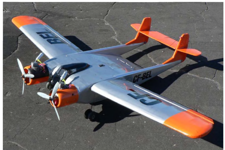
Photo7: This was Flaps' twin CBY-3. It was easy to find the CG on a model of a full scale design because the center of lift of both the wing and the fuselage airfoil are located at the same point. We balanced between 25%-30% back on the wing and it flew great.
