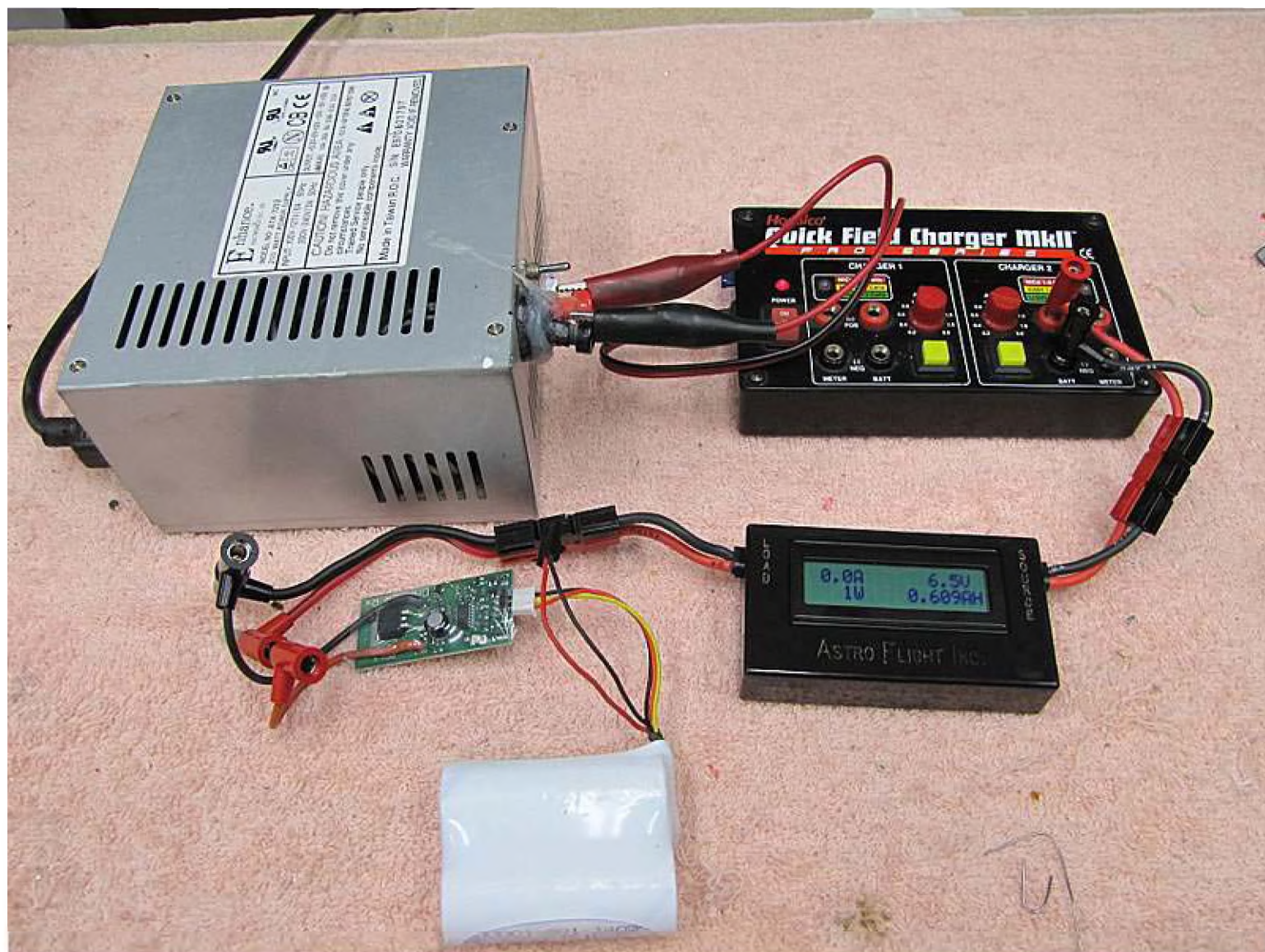
Photo 3: Recharging the A123 battery and recording the results.
