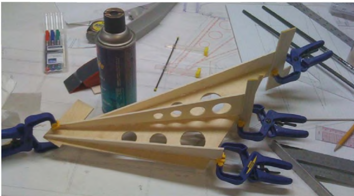
Photo 2: The main float center former with the rest of the structural formers being clamped in place while glue cures. Note the use of Balsa plates at top of strut to keep both former halves at 90 degree angle to main former.
