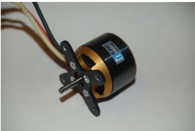
Photo 1: One of the big reasons that outrunner brushless motors such as this are so popular is that they can reap the benefits of spinning big props without the need for a gear drive.
