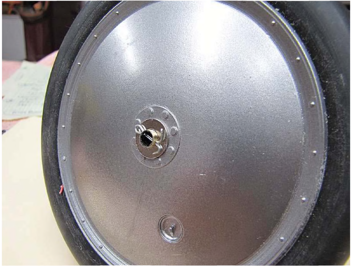
Photo 10: And, here's the wheel mounted with a cotter pin
