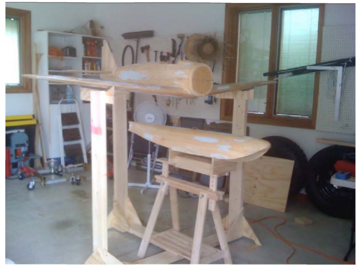
Photo 6: Jig horse built to aid in alignment of fuse to main float. The lower part also is used to hold the model after it is assembled. Notice adjustability in the float stand for proper alignment to the fuse datum line.
