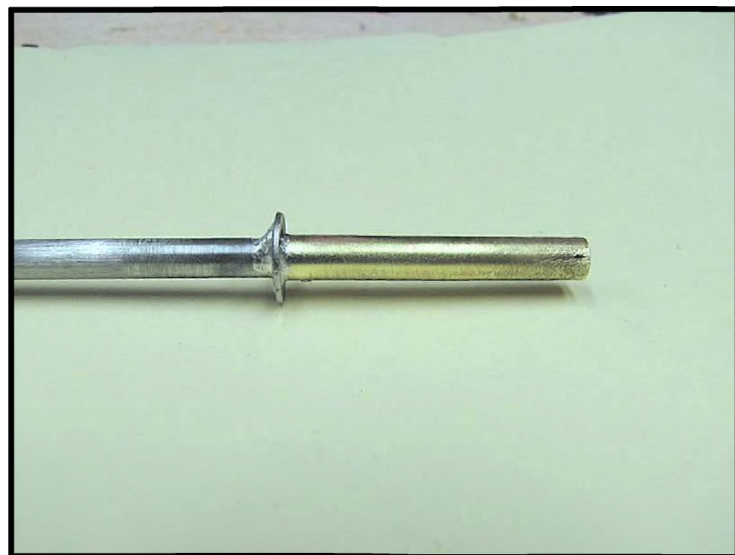
Photo 9: Here's what the axle looks like after soldering
