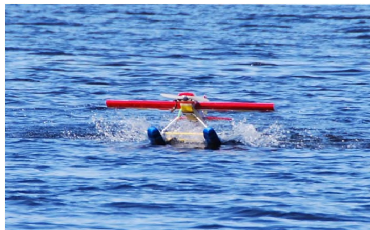
Photo3: This is Ed's Stinger 40 ARF with Plane Fun Floats, U-Can-Do gear for struts and Saito .91 power. Yes. It's a dead stick. Can you see why? Note the green pressure line hanging down. The pressure fitting vibrated loose, and then stripped out the muffler. No muffler pressure and you'll usually get a dead stick.
