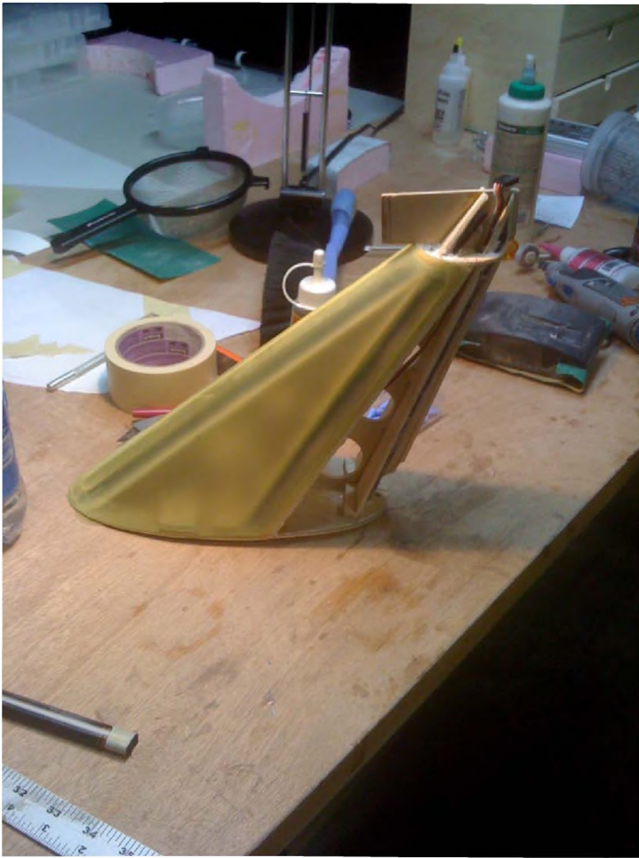
Photo 4: Depicts the skinning process of the main strut using Flight Skin. You can also see the rudder servo lead extension, along with the ¼" mounting plates.
