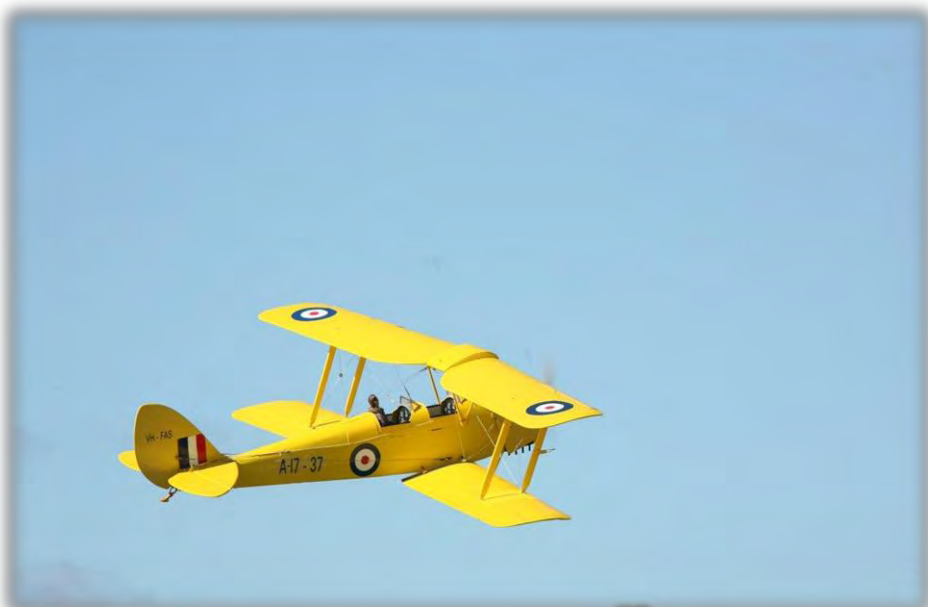
Tiger Moths have a fuel tank on top of the wing center section - perfect for gravity feed.
