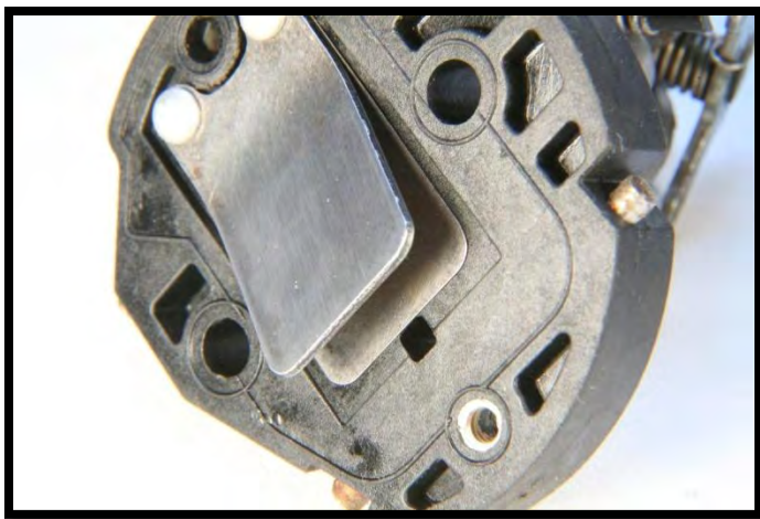
This reed block is after the carburetor in a reed valve engine. The flat plate is the stainless steel 'reed' and the curved plate is the reed restrictor.
