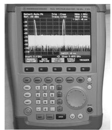
Photo 3: Spectrum Analyzer set up to view frequencies 2.40-2.4835 GHz. The two spikes are the frequencies chosen by a single Spektrum DX7 transmitter.
