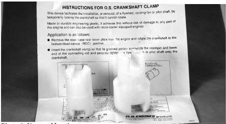
Photo 6: You could make stop tools like this using a wooden dowel if you have a regular use for them.
