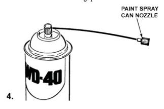
4. Don Madison, of San Diego, CA, has found still another way to keep spray can nozzles unclogged and ready to go the next time they're needed. He lightly sands the end of the red plastic tube that comes with WD-40 cans, until it fits into the bottom of the spray nozzle. When finished spraying paint, a quick squirt of WD-40 will remove any paint residue left in the nozzle. The whole procedure takes only seconds, and
