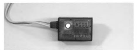
Photo 4: Spektrum Flight Log display shows H000 here, indicating no holds. mitters would cause a ground range reduction. (Most radio manufacturers recommend keeping all internal wiring well away from the receiver antenna(s) in our models, and we made every effort to do so.)
