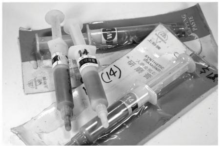
Photo 2: Diamond paste comes in three grades. I find the course or medium most suitable for our type of work. It's inexpensive and available from tool stores.
