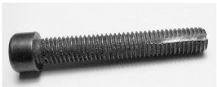
Photo 1: Homemade thread cutting tap made from a common bolt, by cutting the slot at the end, as seen here, with a moto-tool cutting wheel.
