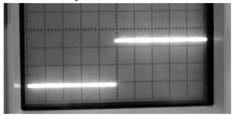
Photo 2: "Response time" as viewed on the oscilloscope. Oscilloscope is set up at two volts/division (vertical) and five millisecond/division (horizontal). The landing gear switch was operated which triggered the trace to start moving across the screen. The jump to five volts (from servo amp circuit output) occurred in about five divisions or 25 ms.
