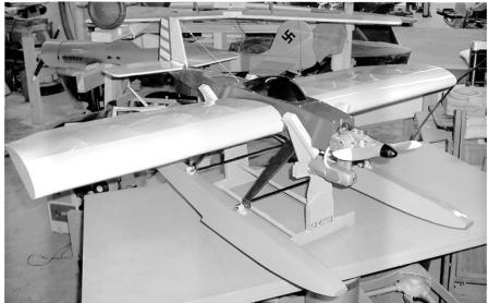
Photo 3: James Welch's Uproar on floats is powered by an O.S. .46AX, and is waiting for spring to test on the lake.
