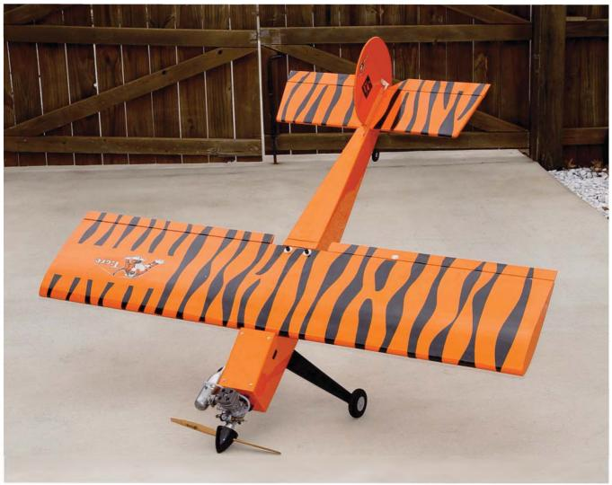
Photo 1: My "Tiger 90 Stick" came from a 1986/7 vintage Modeltech ARC "Joss Stick" kit. Completed and ready to fly at last, it sports an equally old Supertigre S90K engine, but a new Spektrum flight pack commanded by a Futaba 10C radio with a Spektrum RF module. I used a hokey ol' wooden prop for engine testing at home, but it will fly with an APC 14x6 when the time comes.
