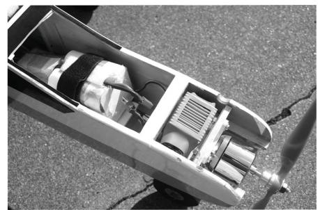
Photo 2: With the battery hatch removed, we get a good look at the 6-cell A123 battery that occupies the space once taken by a glow fuel tank. Also notice the unplanned yet ideal mounting spot for the ESC just behind the motor. While not elegant, this location will provide a nice source of cooling air.
