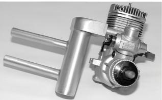
Left: With one extension, the O.S. .46AX muffler will work, but the cowl will require more cutting, and the firewall will have to be modified. At right is the \$36 Bison Pitts-style muffler. It makes assembly easier, and makes the completed model look nicer. I later shortened the tubes by about half. The noise level is higher than the O.S. muffler, but is still acceptable.
