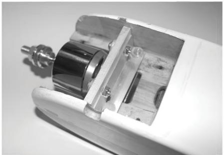
Photo 1: The Grayson Hobby GH3520-12 motor gives a little over 600 Watts for this 6 lb. airplane, perfect for my 100 Watts/lb. target. The aluminum X-mount included with the motor required some reshaping to fit the motor cleanly. Some aluminum angle stock and 1/4" lite-ply was all it took to mount an outrunner brushless motor to the existing beam mount of the Minicraft Simpli-Fly 40.
