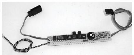
Photo 1: Circuit built to aid in measurements of "response time". This circuit is basically a servo amplifier (right) with an opto-coupler and a chip (left) to clean up the pulses. This circuit plugs into the receiver's landing gear channel, requires its own battery, and the output to be viewed on the oscilloscope comes from the black and orange wires.
