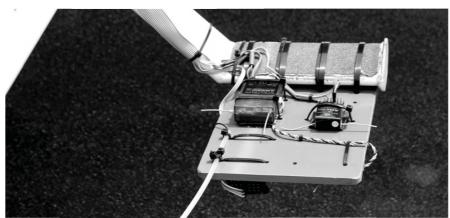
Photo 7: The test platform was mounted to the loading step of a Cherokee Six airplane, with the three receivers. Note the tube for the 72 MHz antenna.
