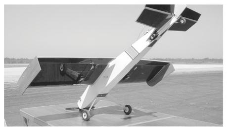
Photo 2: Ed's Little Stick with downward end plates to stop roll with rudder. anhedral. Photo 2 shows my Little Stick with downward end plates.
