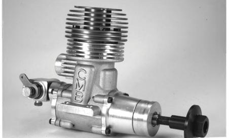
Photo 7: This CMB 80 ducted fan engine has the potential to rev very high with a fan or flywheel, but it still runs very nicely with applicable size normal props, which is what I used when I tested it for a review.
