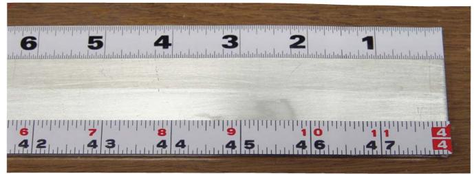
Photo 3: Here you see what used to be the blank, backside of my 48" measuring stick. Using stick-on measuring tapes, however, I converted the useless blank side into a useful tool.
