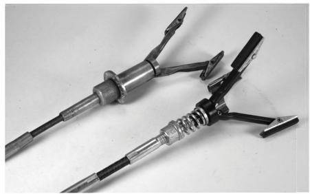
Photo 1: Brake cylinder hones are ideal for honing model engine cylinders.
