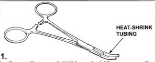
1. Steve Cross, of Wildwood, MO, uses medical forceps to remove and replace fuel lines when filling some of his fuel tanks. Over time, he found the teeth on the forcep jaws damaged the fuel line, sometimes causing leaks. He resolved the problem by placing heat-shrink tubing over the jaws. They still grip well, but no longer bite into the fuel line tubing. Short lengths of silicone fuel tubing would also work.
