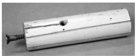
Photo 3: Here's a simple wooden lap that works well. Drill a hole through the end of the slit to prevent it from breaking as you wind the screw in.
