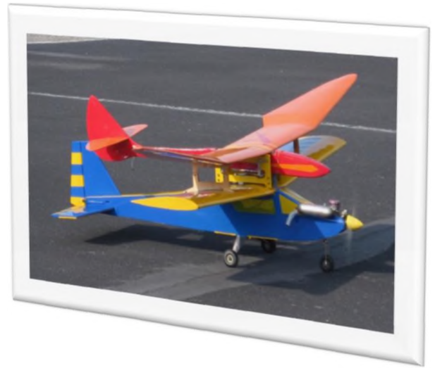
Carlos Reyes' Monster QB-60, glider lift plane shown carrying a Bird of Time. It's powered by a Tower .75. This is a Pilot kit from the 1980s. The glider mounts and hardware all came in the kit.
