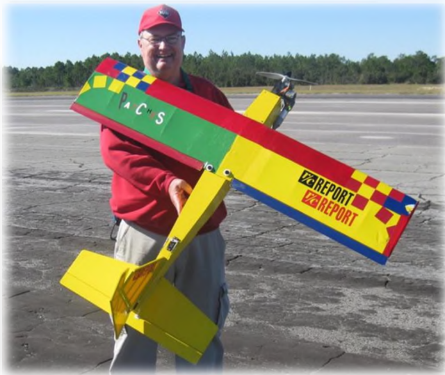
Ed & Patches, an original Stick-type plane constructed from a modified World Models Skyraider Mach I wing that has one rib removed from each side and 3 degrees of anhedral.
