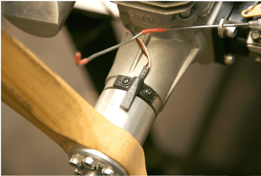
Photo 7: Orientation of the sensor is important, as it must be in accordance with the polarity of the magnet exciter in the propeller hub.
