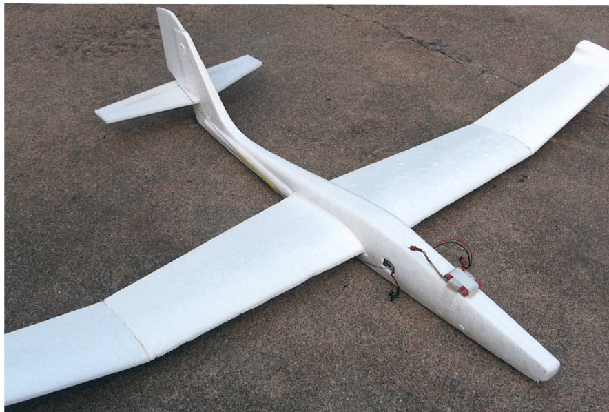
Photo 6: No need for a high-end molded glider here. A $5 'chuck-it glider' converted to R/C provides plenty of low cost fun.
