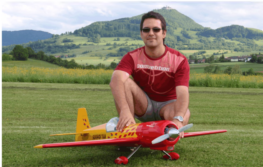
Photo 2: Jorge Estrada with his Su-31. Jorge uses a Thunder Tiger .75 4-stroke in it. He originally had trouble with the engine leaning out and quitting, but found he had fuel foaming. With a little extra foam around the tank, the engine turned out to be a sweetheart.
