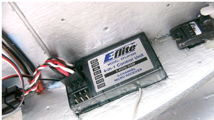
Photo 2: I was hoping that the differential-thrust yaw control inherent to this heli 4-in-1 unit would have more control authority, but even so, the Lil-Lightning is still a hoot to fly in calm airs.
