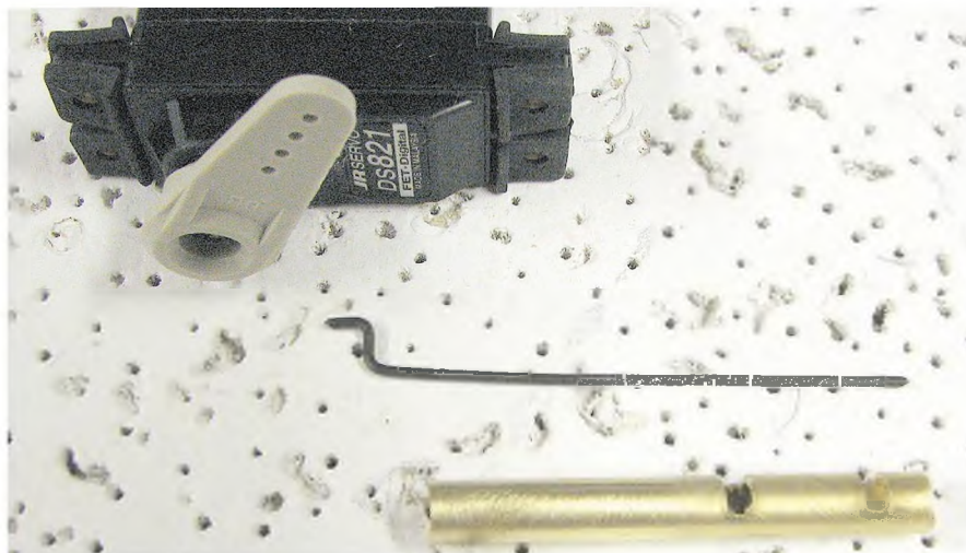
Photo 3: Parts of release mechanism inside fuselage
