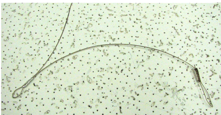
Photo 8: Details of front end of tow lead showing two loops
