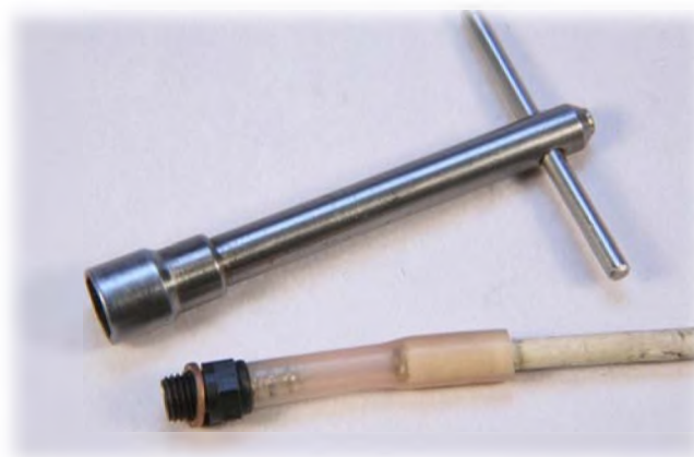
Photo 4: A short length of fuel tube on a wire handle makes the safe plug insertion tool. The spanner is a fancied up cap head bolt with a 2" handle.
