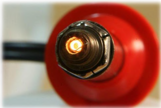
Glow plugs should glow brightly and almost for the full length of the element.
