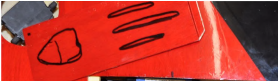
Photo 1: Note the cooling holes marked in the bottom of the battery tray and on the hatch cover. Just quick and dirty with a felt marker!
