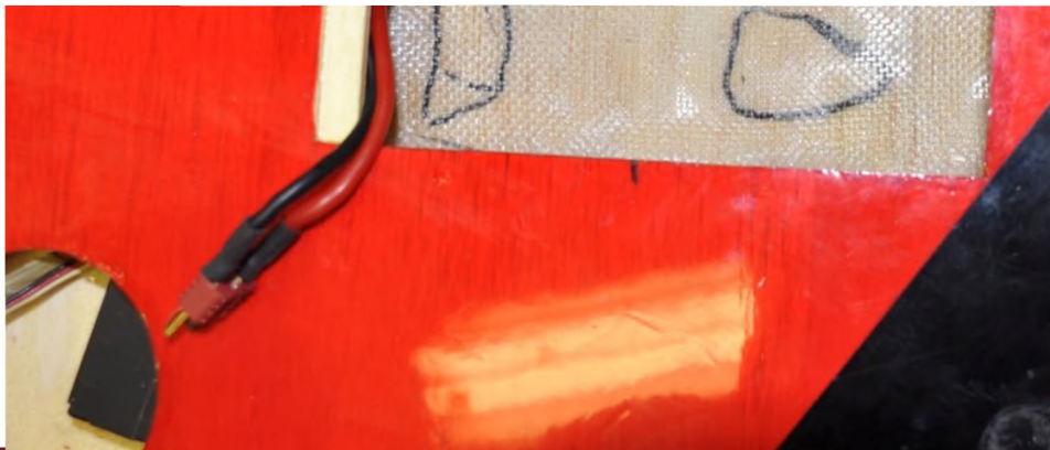
Photo 1: Note the cooling holes marked in the bottom of the battery tray and on the hatch cover. Just quick and dirty with a felt marker!
