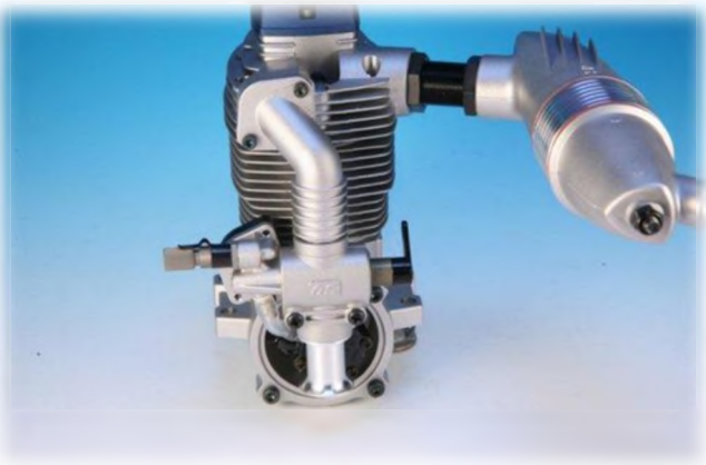
The pump and carburetor neatly packed behind the engine away from harm.
