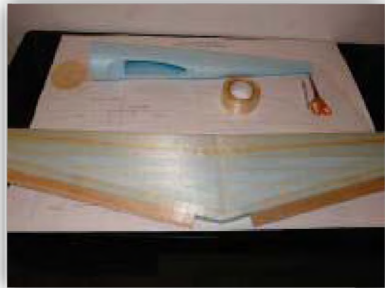
Photo 6: Wing covered with BiDi Tape and Ailerons attached
