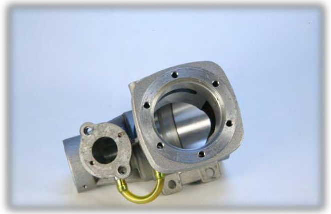
Well cast, finely finished maincase. Note the Tygon connection from the transfer passage to the intake manifold to drive the fuel pump.
