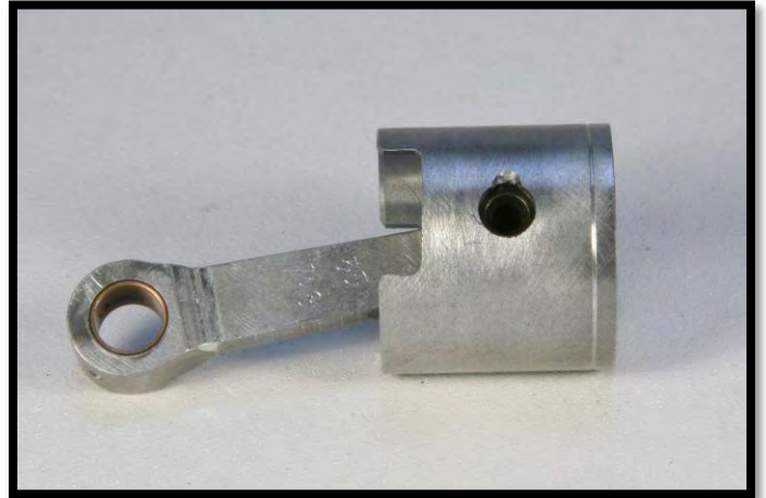
The machine marks on the piston are from the honing process to ensure perfect roundness.
