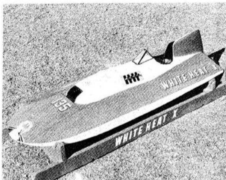
Typical high-speed hydroplane fitted with O&R 1hp motor.
