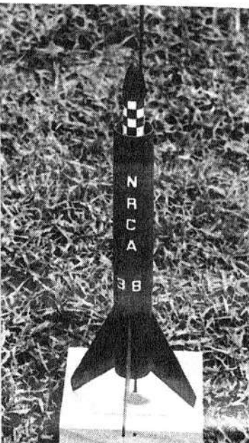
BELOW: A Jet-Pump rocket. This highly efficient model makes use of the ramjet system of propulsion.
