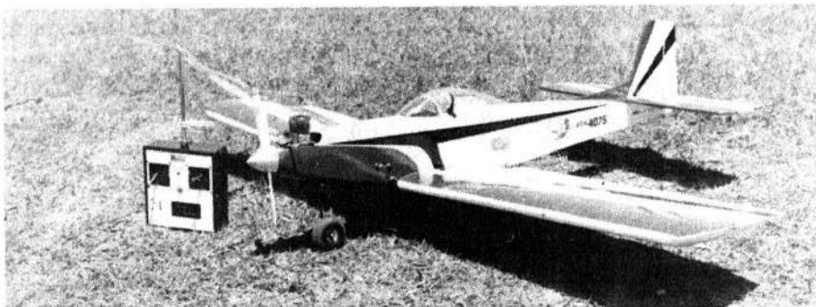
NICELY finished Beachcomber by L. Winly. Powered by Enya 60, it weighs in at 6½lb. Silvertone RX.
