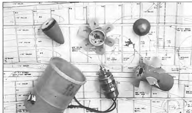
An EDF-700 dismantled. Top centre is a six blade rotor, next clockwise are stator fixing screws, spinner, motor tube with stator blades, 700 motor with prop adaptor fitted, fan housing (shroud) and last, the tailcone.
