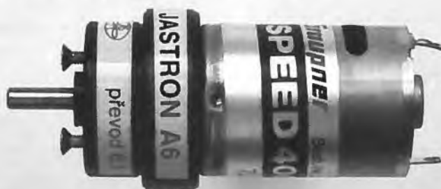
Jastron A6, 6:1 ratio gearbox on a Speed 400 motor.
