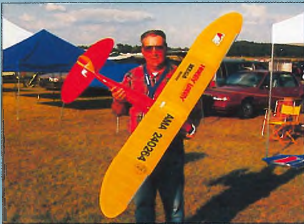
Jay Burkart with Playboy Pylon winner of LMR event, MEGA Mini with Kruse 2 to 1 gearbox, Aeronaut 14 x 7 prop set not to fold.
