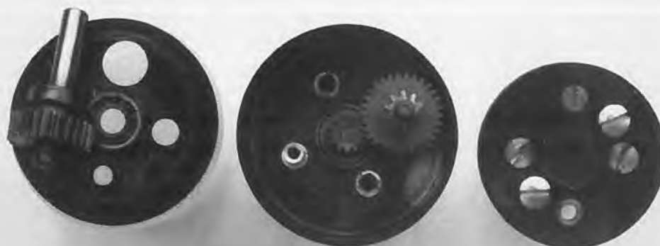
Jastron A6, 6:1 ratio gearbox on a Speed 400 motor.
