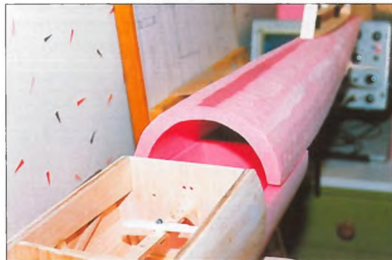
The bottom and nose is made of pink foam that has been hot wired and sanded to shape. After this the fuselage sides were sheeted with 3mm balsa.
