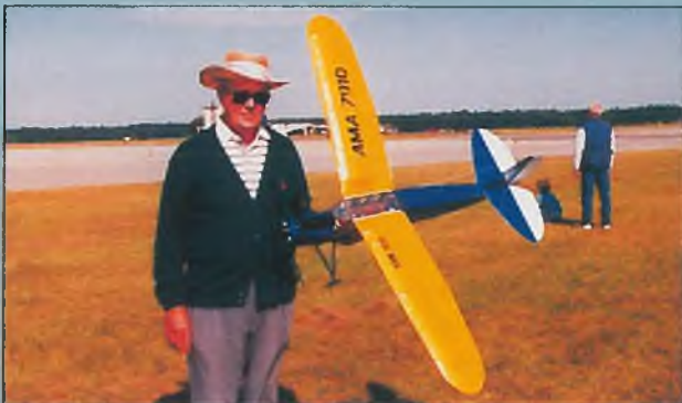
Pat Harrison with his Lanzø scale Puss Moth, Spirit of SAM event, Graupner Speed 400 with Graupner 6 to 1 gearbox, Master Airscrew 15 x 12 prop.
