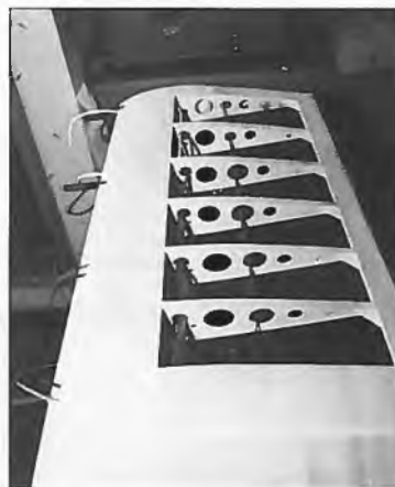
Half the wing centre panel with lightened ribs. You can just see the black carbon fibre tubes for each motor nacelle, wiring to the motors and servo lead.
