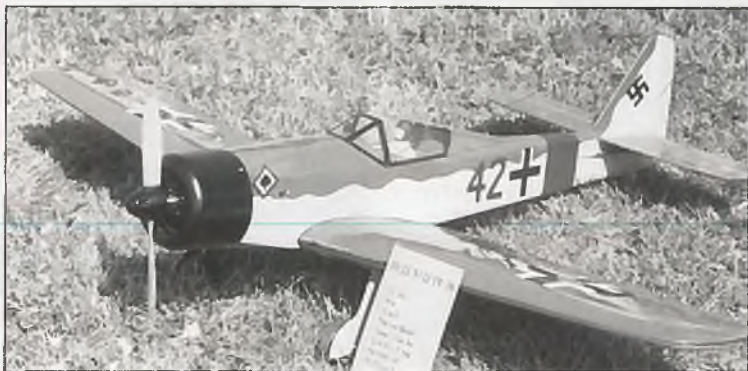
The stand off scale FW 190 was brought by Gary Grollmund. Originally a Wing Manufacturing "short kit", it has a 54" span and an all up weight of 94 oz. for a wing loading of 20 oz/sq.ft. Gary powered the model with a custom 2:1 twin gear box using a pair of "Green Machine" car motors. It had 14 x 1700SCRCs and a 12 x 10 Master Airscrew electric prop. (These are great props for gear driven motors. They are heavily undercambered so aren't much use over 6 or 7,000 rpm, the same way undercambered wings are best on slow airplanes, having too much drag to go fast.)
