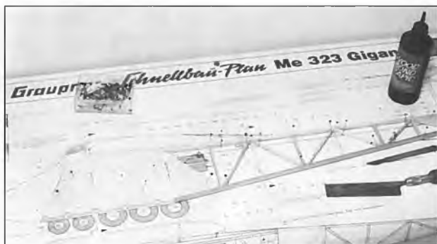
The fuselage is just a box made from spruce longerons and balsa uprights and diagonals.
