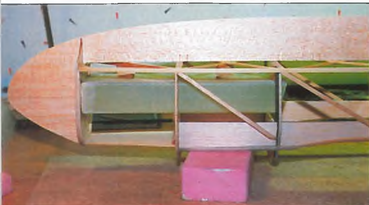
Integral with the fuselage frame is a fibreglass tube for the battery, which is slid along the tube until the CG is correct and then fixed.
