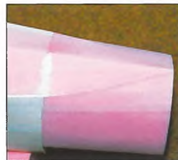
The bottom and nose is made of pink foam that has been hot wired and sanded to shape. After this the fuselage sides were sheeted with 3mm balsa.
