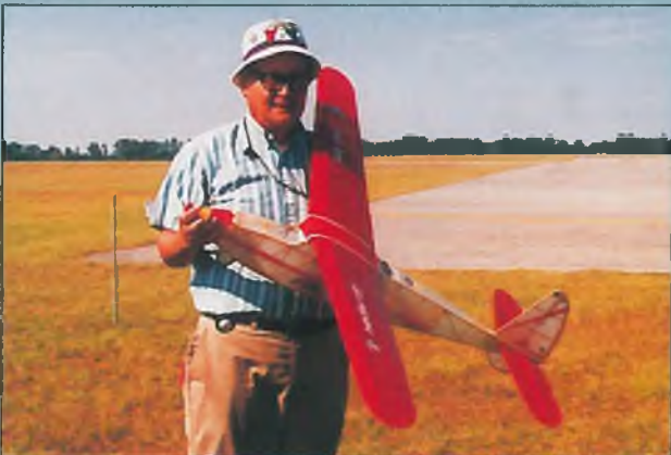
Dick Huang with his Comet Phantom Fury, Spirit of SAM event Graupner Speed 400 with Master Airscrew 6 to 1 gearbox, Geist 14.75 x 7.5 prop.
