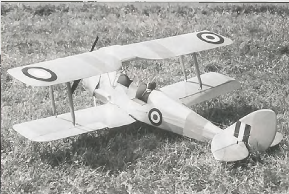
Thayer Syme built a lovely Tiger Moth from the Gordon Whitehead plan. It has a 47 1/2" span and a wing area of 631 sq.in. Thayer lightened the ply nose section and used contest balsa throughout. With an Astro geared FAI 15 and 10 x 1700SCRCs, the 12 x 8 prop draws 26 amps and gives flights in excess of 5 minutes.
