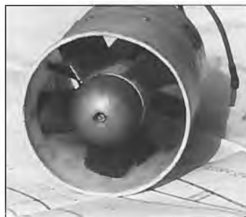
A five blade EDF-700. You can see how close a fit are the rotor blades to the shroud.
