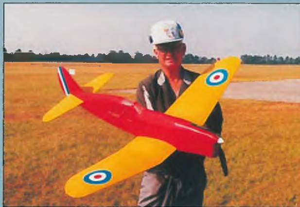
Eut Tileston with his Stahl design scale Caudron Fighter flown to sixth place by Kirby Hinson in Spirit of SAM event. Graupner Speed 400 with Simprop 5.9 to 1 gearbox, Master Airscrew, 15 x 12 prop.
