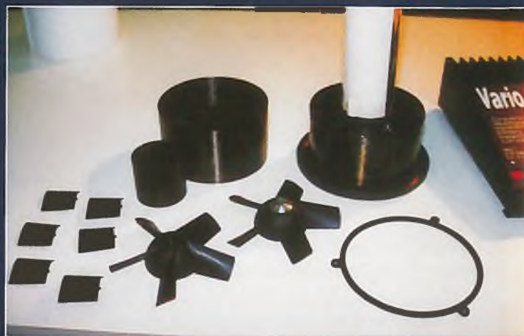
Aero-naut Turbo-Fan 1000 with carbon reinforced shroud. The one on the right shows the long motor tube.
