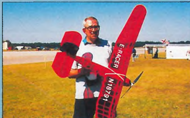
Jack Hiner with his Lanzo Racer placed second in Texaco event, Leisure 28T with Leisure 3.8 to 1 gearbox, Aeronaut 16.5 x 15 prop set not to fold.
