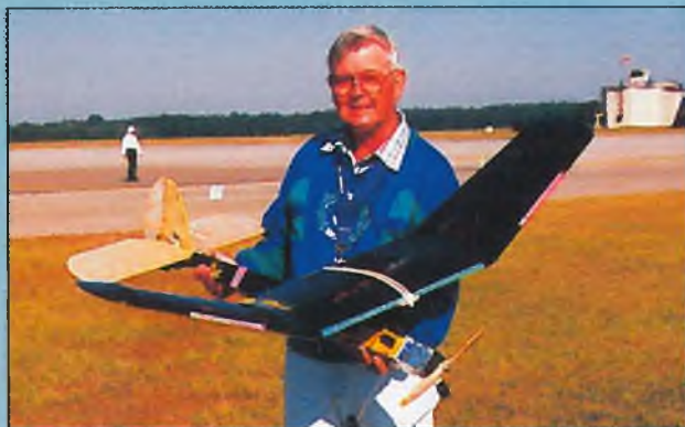
Jerry Smartt with his Lanzo Bomber placed third in LMR, Trinity 16T with Master Airscrew 3.5 to 1 gearbox, 11 x 7 Master Airscrew wood prop.
