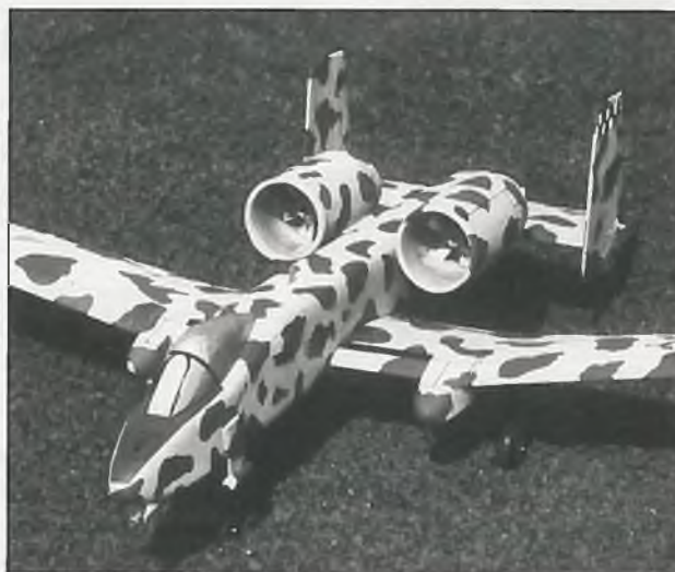
Gernot's A-10 uses two EDF-600 units and eight cells.
