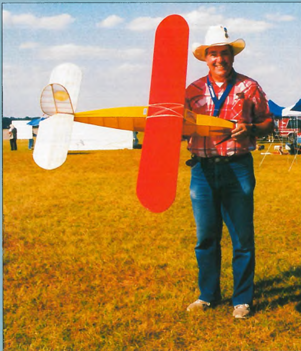
Jay Burkart winner of the Spirit of SAM event with Lanzo Cabin, Graupner Speed 400 with Simprop 5.25 to 1 gearbox, Aeronaut 13.5 x 8 prop.
