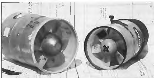
The size difference shows here, the 700 is almost twice the weight of the 600 for more than twice the thrust.
