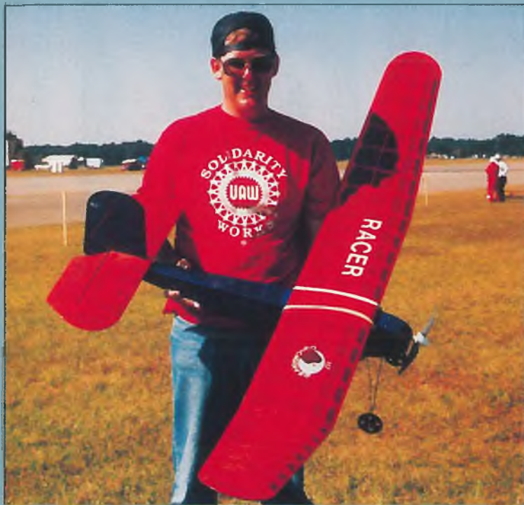
Michael McIntyre with his Lanzo Racer, Mike was using the newly developed Astro Texaco 035 motor with a Leisure 2.43 gearbox, Aeronaut 16.5 x 15 prop set not to fold.
