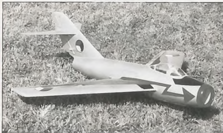
The Mig 15 was built by Dave Ribbe and has appeared at a number of jet rallies and contests in the US and Canada and demonstrated to the gas fliers what can be done with electrics. It has a 56" span and a wing area of about 4 sq.ft. The motor is a 6 turn Astro 40 on 18 or 20 x 1700SCRCs turning a modified Viojet rotor clipped to 4.2" dia. It draws 50 amps static but with a little throttle work he gets 3 1/2 minutes in the air. It is equipped with retracts and weighs 6 1/4 lb. Flights were quite impressive with good speed and adequate vertical, probably better than the original. I know of at least two other pilots who are starting on their own versions of this model.
