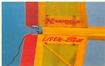
▲ Tail surfaces can be unplugged anytime.
