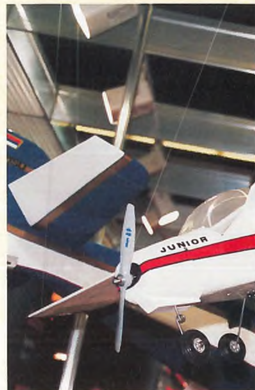
▲ Graupner 'Bölkow Junior' for Speed 4006V FG 1.85 and 8 x 500AR cells. Span is 1 metre (39").
