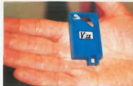
▲ The new 10mm thick servo for installation in wings and fins. The frame is built into the wing and actually strengthens it. The 'box' on the base permits egress of servo cable (this is just an empty case).
