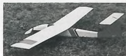
▲ Author’s much modified Ridge Runt provided an excellent introduction to modern ‘soft’ electric flight. Speed 400 7.2V, 2.33 gearbox, Aero-naut 9 x 6.5, 8 x 800AE & Jeti 10.
