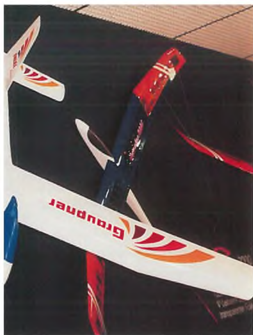
▼ Simprop Ventura, 2650mm (104") wingspan, moulded fuselage, moulded veneered wings with ailerons. Recommended power is Power Speed 2000-7 with 3.25:1 gearbox and 8 x 2000mAh cells.
