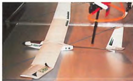
▼ Hirobo G-22VM. One of four G-22 aircraft, with cruciform or V tail and glider or electric.
